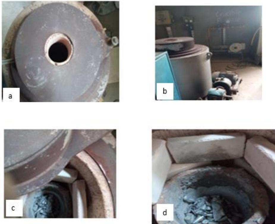
**Plate 1:** Crucible Furnace: Cover (a), Furnace (b), Furnace lined with Researched Bricks (c-d)
