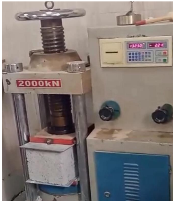
Figure 2: Crushing of Block using the Universal Compression Machine
