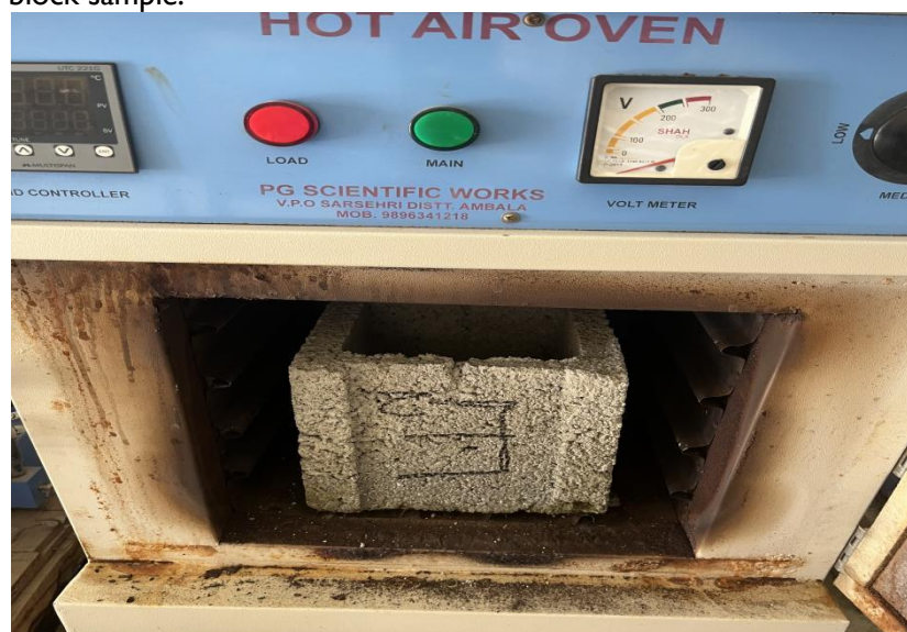
Figure 3: Block samples oven dry in oven for 24 hours
