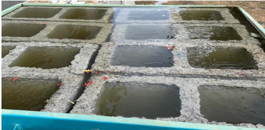
Figure 4: Sandcrete Hollow Blocks immersed in Water for 24 Hours
