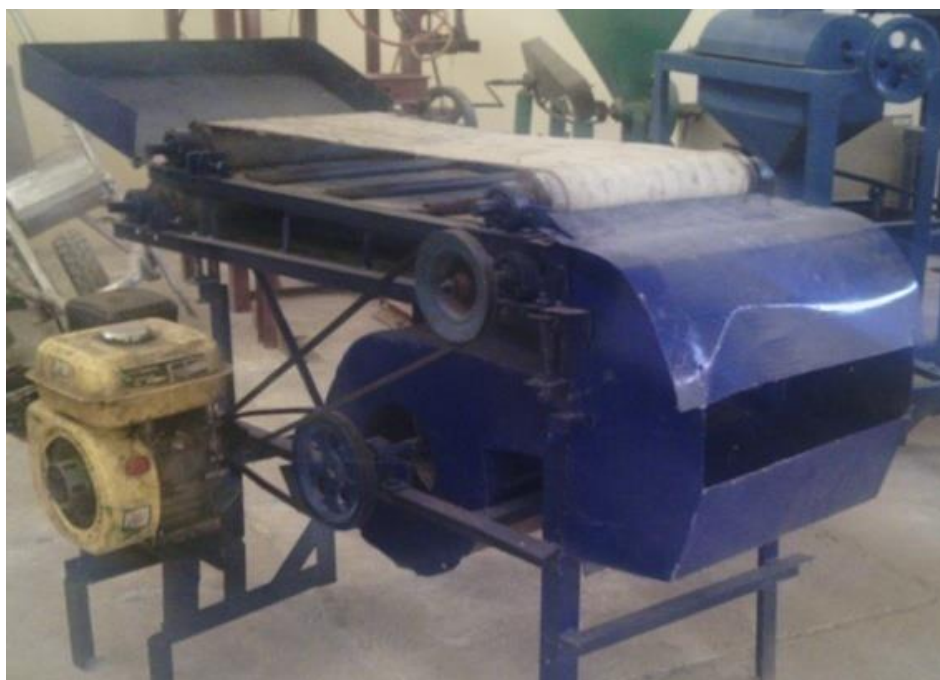
Plate I: The constructed isometric view of the canvas belt cowpea thresher
