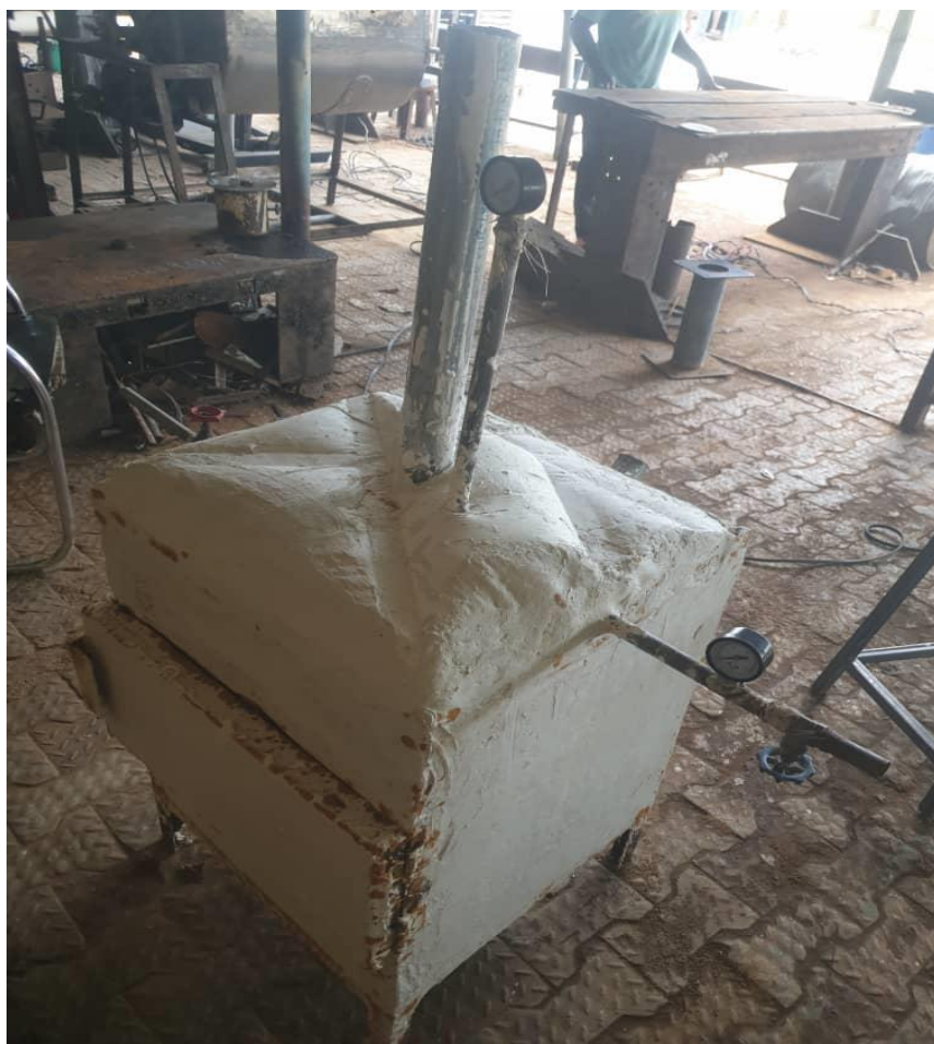
Plate 1: Front View of the Constructed Batch MSW Incinerator
