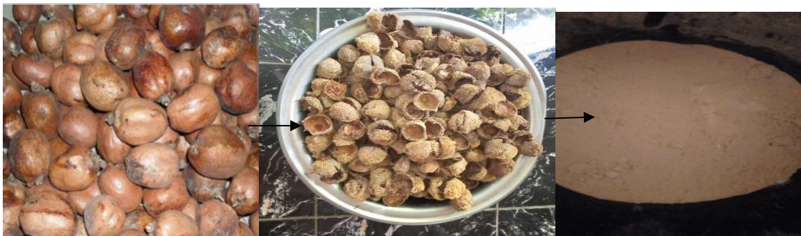
(a) Doum Palm fruit (b) Doum Palm shell (c) Doum Palm Particles
