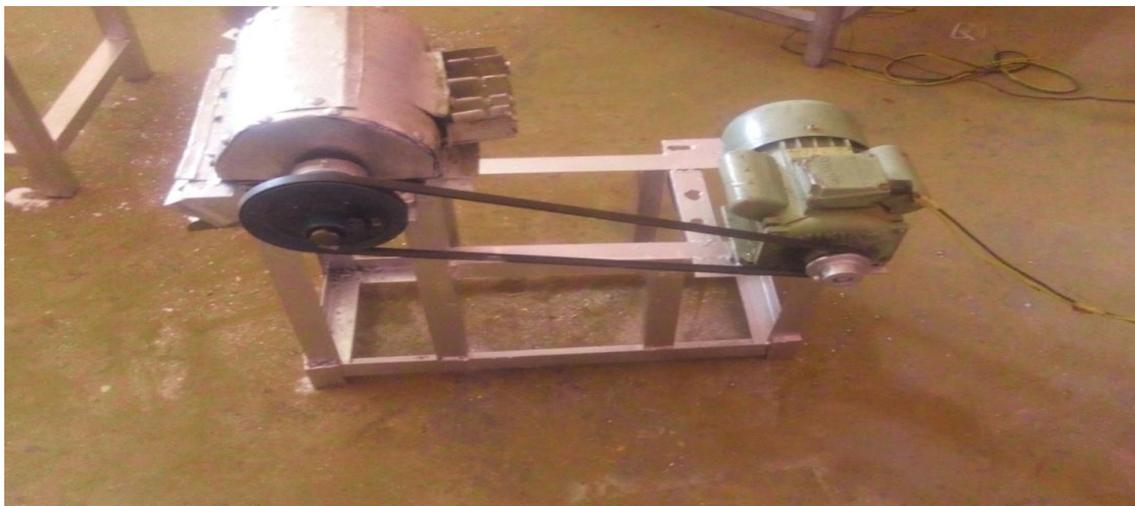
**Plate 1:** Small Scale Okro Slicing Machine.
