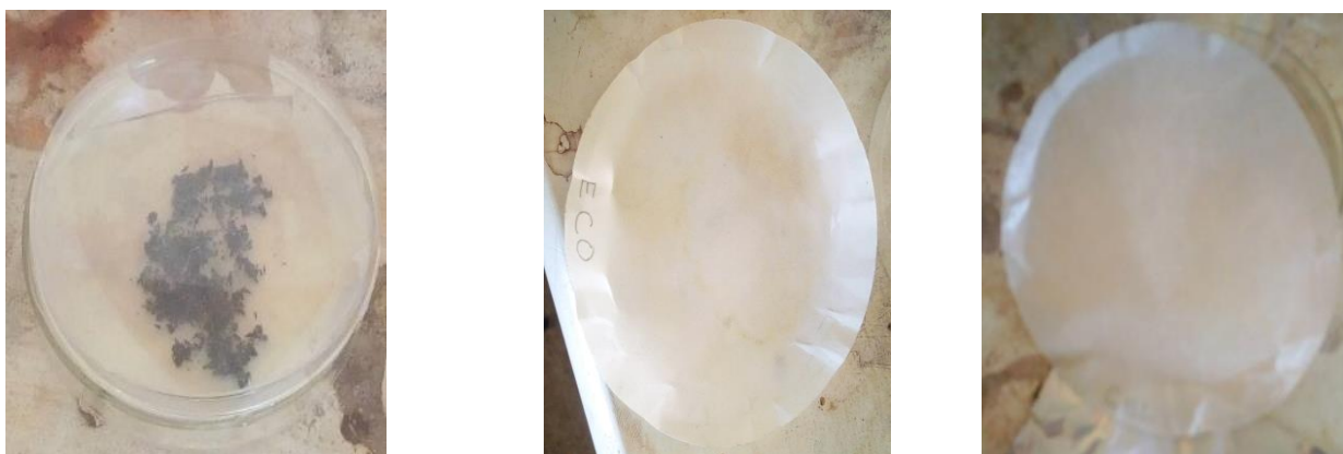
(a) Test with cast iron particles (b) after 2Hrs, castor oil (c) after 2Hrs, SAE 20W50
