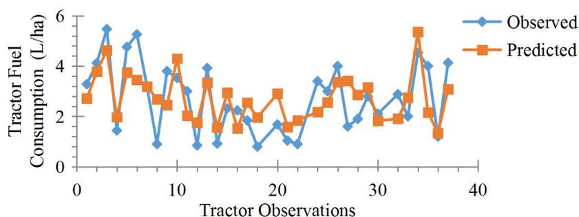
**Figure 1.** The plot of Observed and Predicted Tractor Fuel Consumption using Model 2 of Harrowing Operation
