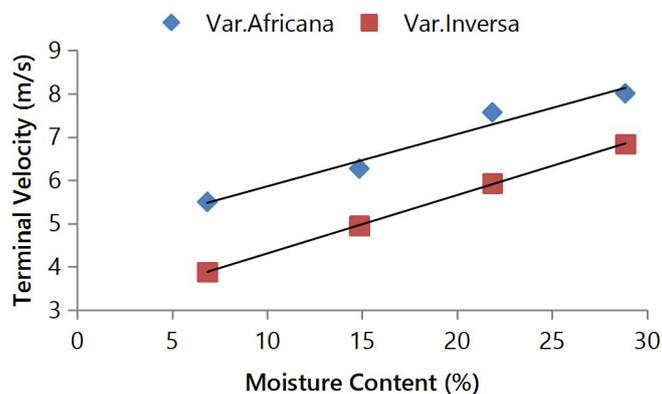
Figure 5: Effect of Moisture Content on Terminal Velocity of Breadfruit Seed Varieties
