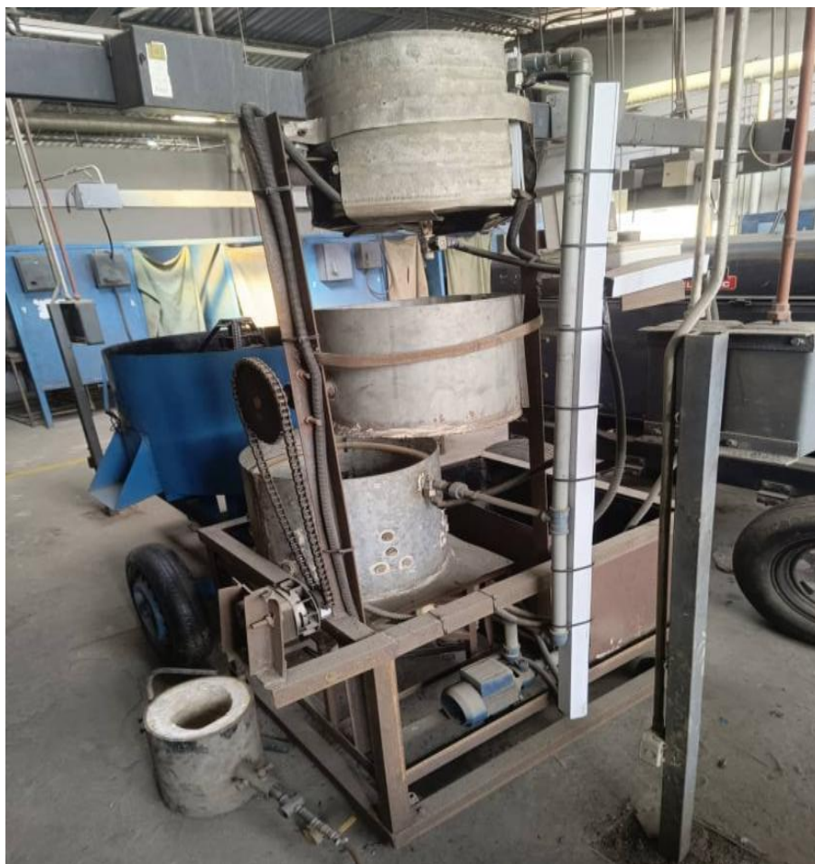
Plate I: Poultry Birds De-feathering Machine
