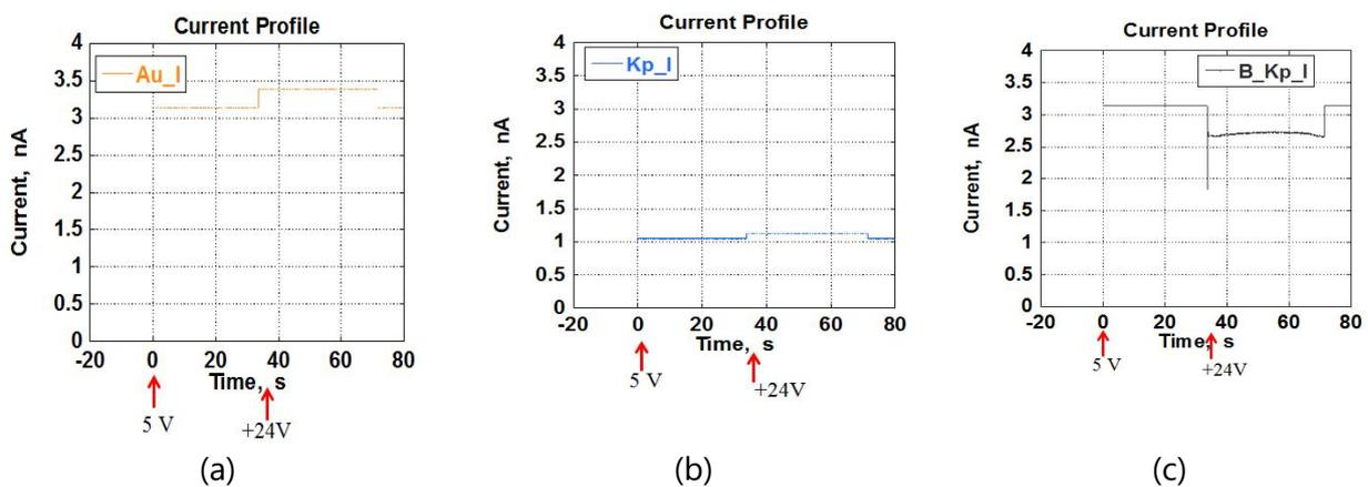
Fig. 8: Samples current profile. a) Gold; b) Kapton®; c) Black Kapton® for on-orbit dat
