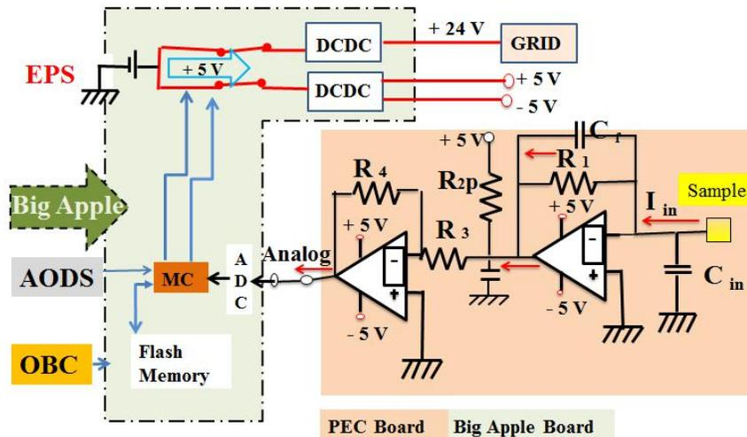
Fig. 5 Schematic diagram of PEC system interfaces (Ewang, 2017)
