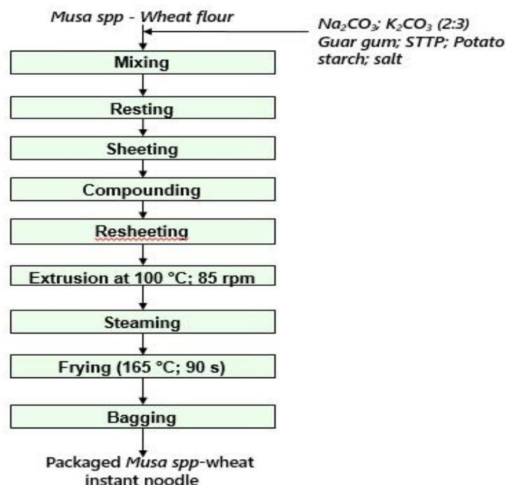
Figure 2: A schematic diagram showing production of fried instant noodle
