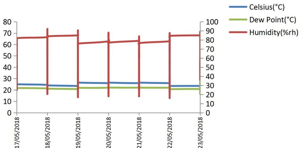
Figure. 2; The Chart of the No Load Test of The Environmental Conditions of the Greenhouse Solar Tent Dryer for Duration of 5 Days
