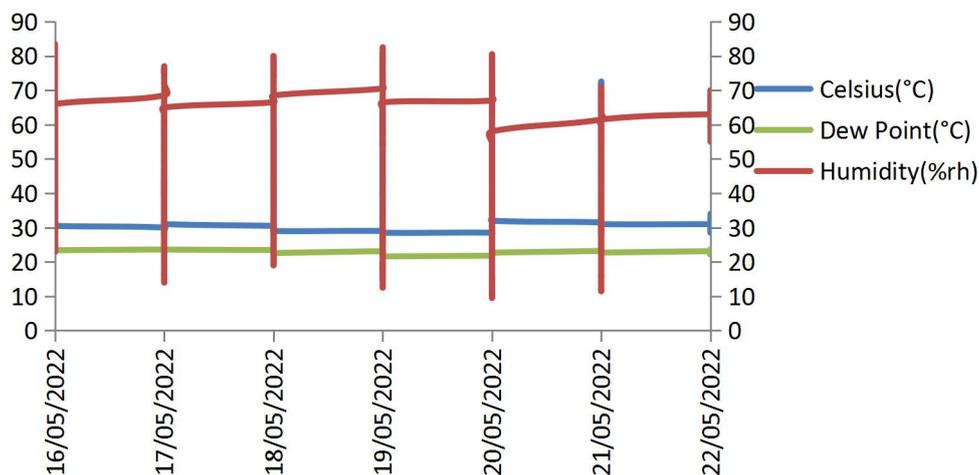
Figure. 3: The No Load Test of the Environmental Conditions of the Parabolic Solar Dryer for duration of 5 days
