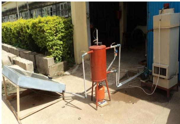
Figure 2: Outdoor components: Solar collector, Hot water tank, gas burner, cooling tower
