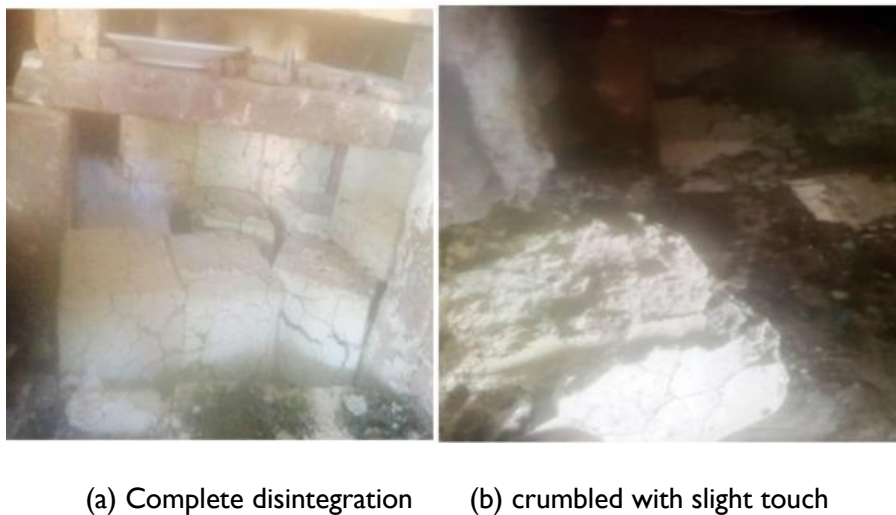
Plate 2: Physical Deterioration of grades BAC at 20% 1000°C
