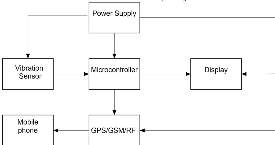
Figure 1: Block diagram of proposed accident detecting device.
