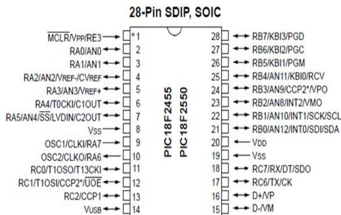
Figure 2: PIC18f2550 microcontroller IC representation. (Microchip 2006)
