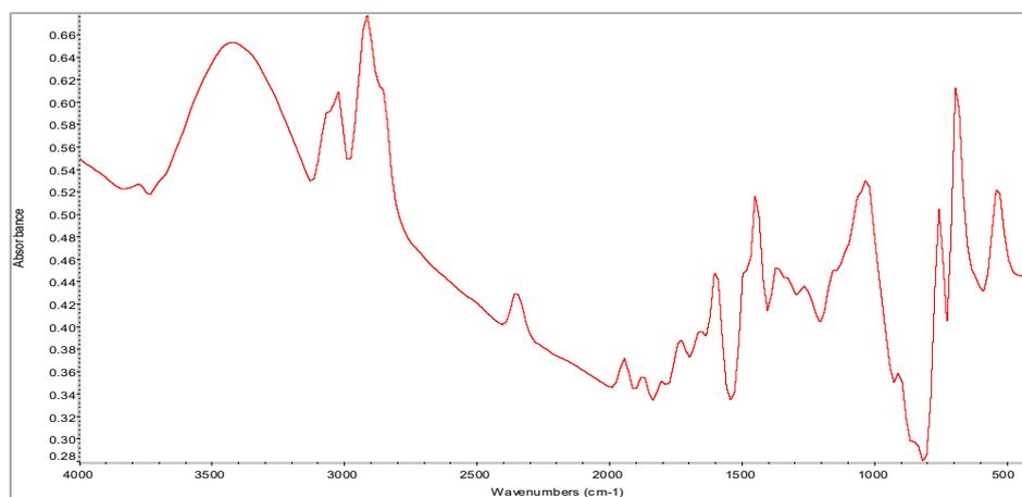
Figure 1: Infrared Bands of Polystyrene based Composites
