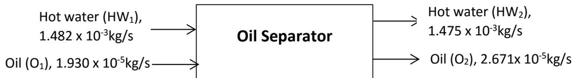
Figure 8: Material balance over oil separator
