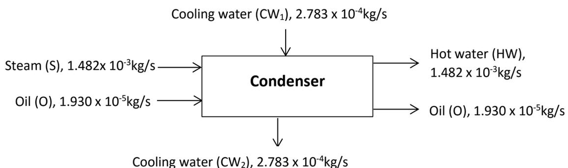
Figure 7: Material balance over oil condenser
