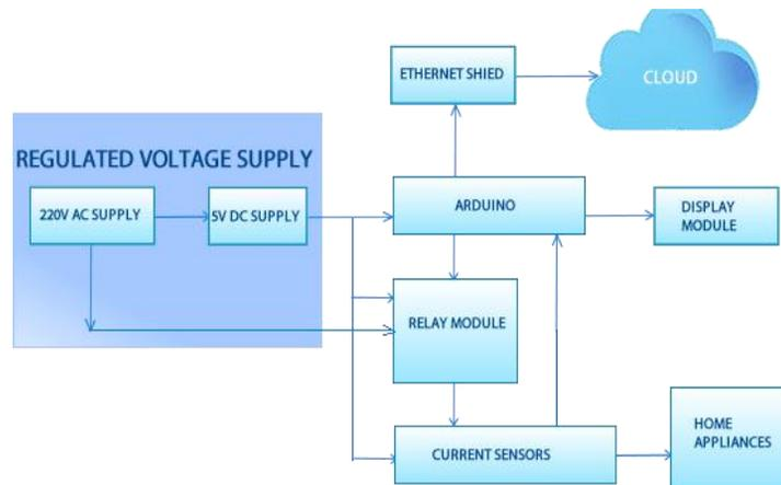
Figure 2: Block diagram of SLCDB
