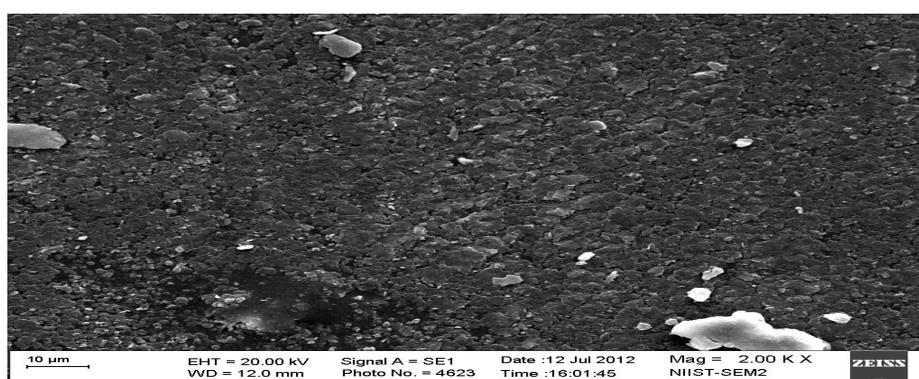
Figure 2: SEM Micrograph for NR/RSO modified kaolin (10 phr)
