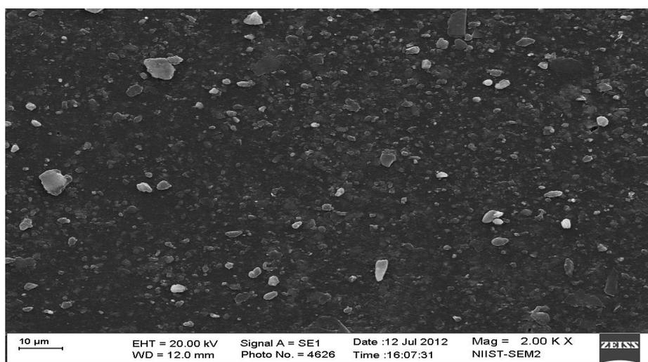
Figure 3: SEM Micrograph for NR/TSO-modified Kaolin (10phr)
