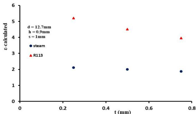
Figure 5: Variations of calculated enhancement ratio with fin thickness
