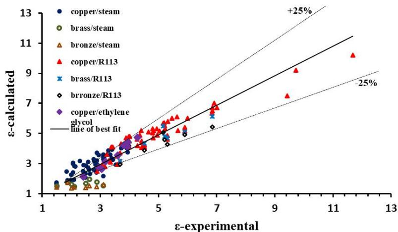
Figure 2: Calculated and experimental enhancement ratios of different working fluids and tube materials
