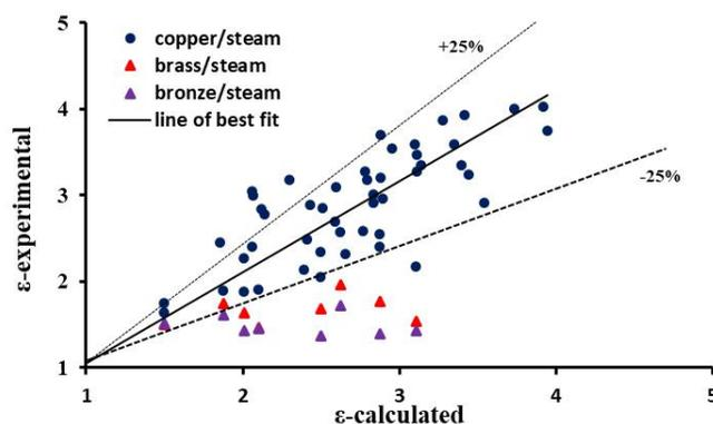
Figure 3: Calculated and experimental enhancement ratios for condensation of steam on copper, brass and bronze tubes.
