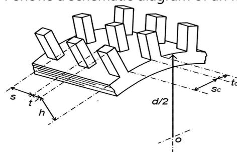
Figure 1: Schematic diagram of idealized rectangular fin-tube (Ali and Briggs, 2013)
