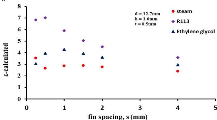
Figure 4: Variation of calculated enhancement ratio with fin spacing ( $s$ )
