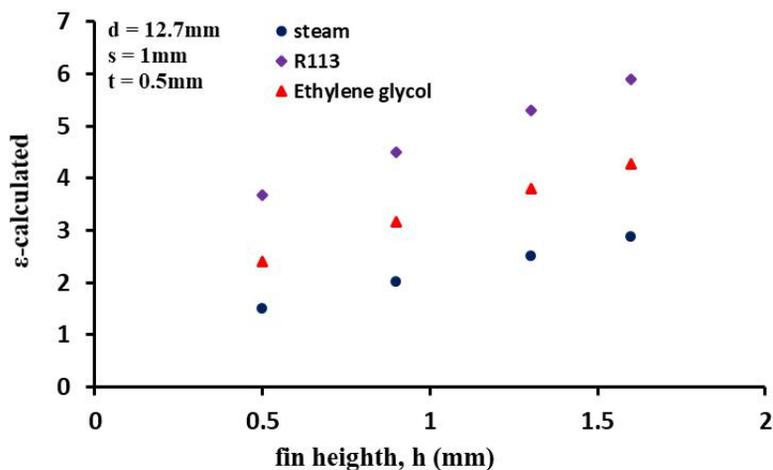
Figure 6: Variations of calculated enhancement ratio with fin height ( $h$ )
