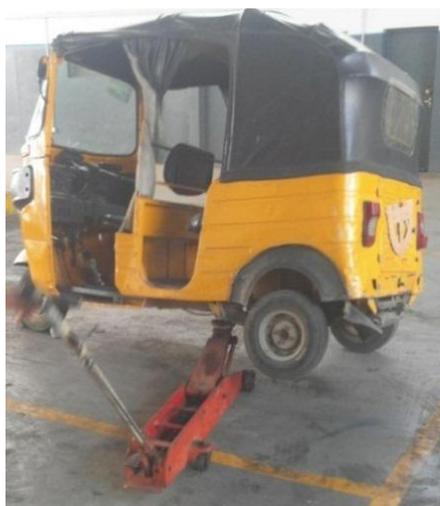
Figure 4: Tilting of TWV to Rollover Angle
