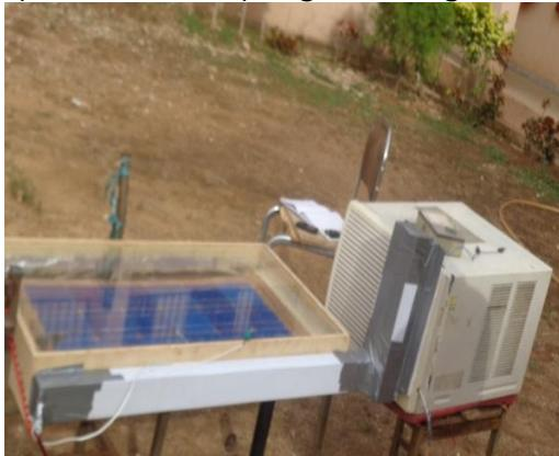
Figure 1: Cooled module
