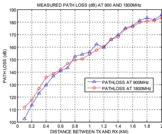
Figure 4: Measured path loss at 900MHz and 1800MHz
