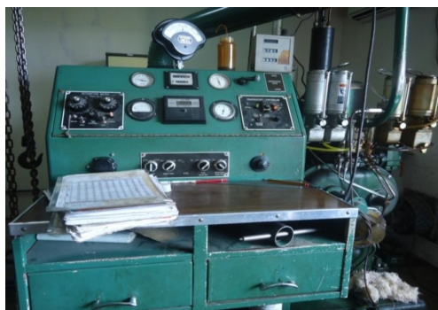
Figure 3: Comparative Fuel Research Engine (C- 48386 model)
