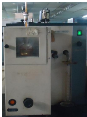
Figure 4: Atmospheric Distillation Apparatus (HDA 620 model)
