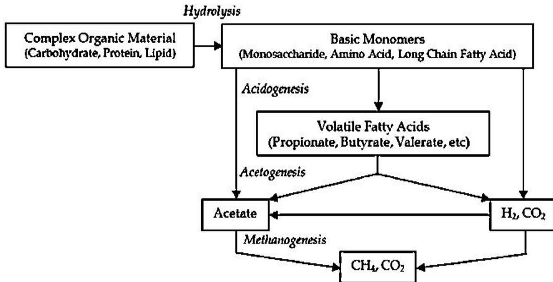
Figure 3. Steps of the Anaerobic Digestion Process (Tauseef *et al.*, 2013)
