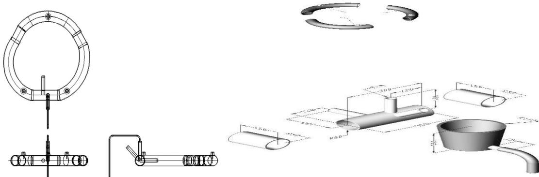
Figure 5. Arrays of the AutoCAD Design of the 12 litres Innertube Digester
