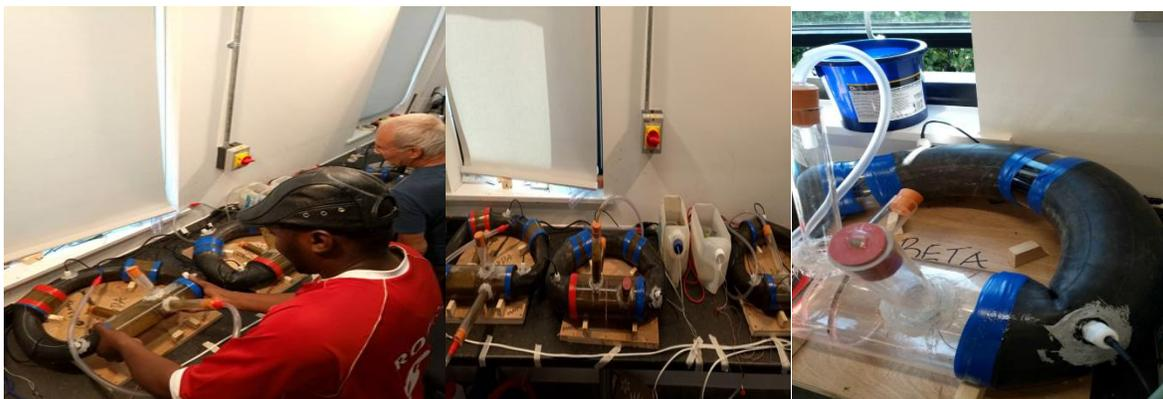
Figure 6. Arrays of the 12 litres innertube digesters been tested
