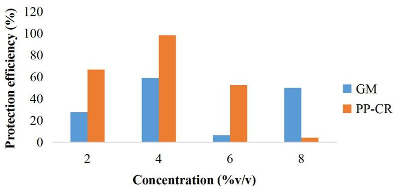
**Figure 3:** Variation of protection efficiency with inoculant concentration for gravimetric based mass loss test and potentiodynamic polarization test.
