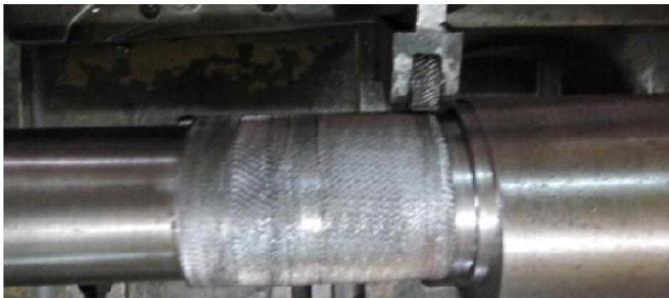
Figure 24: Knurling of the bearing part of the eccentric shaft for force fitting
