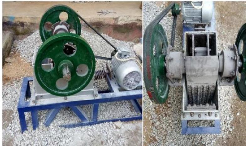
Figure 37: Side and front views of the single toggle jaw crusher
