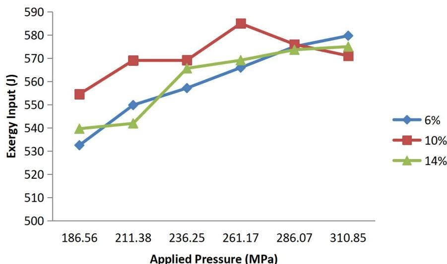
Figure 3: Effect of Applied Pressure on the Exergy Input using Huskdust at Different Moisture Content
