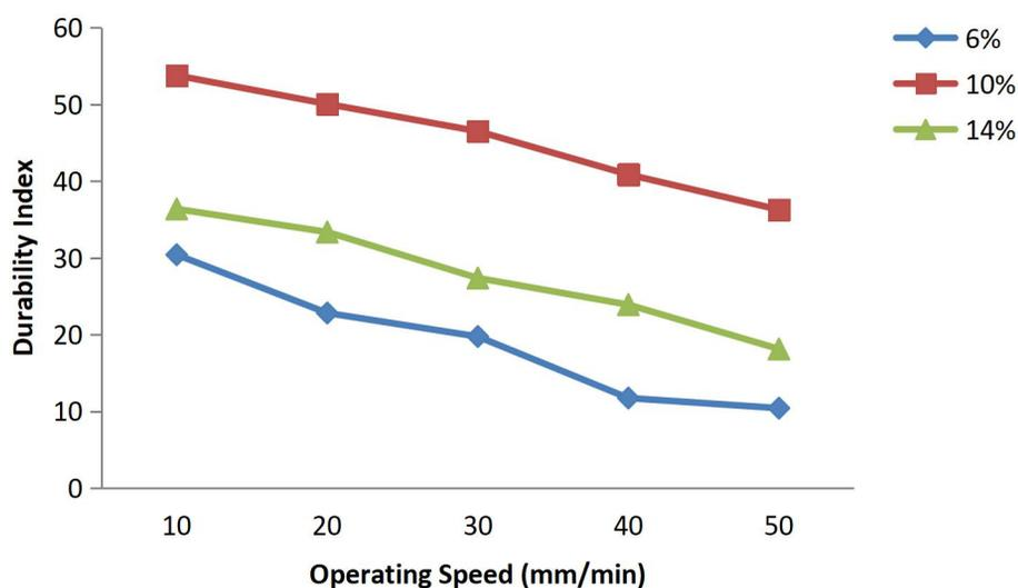
Figure 13: Effect of Operating Speed on the Durability Index of the Densified Biomass from Huskdust at Different Moisture Contents
