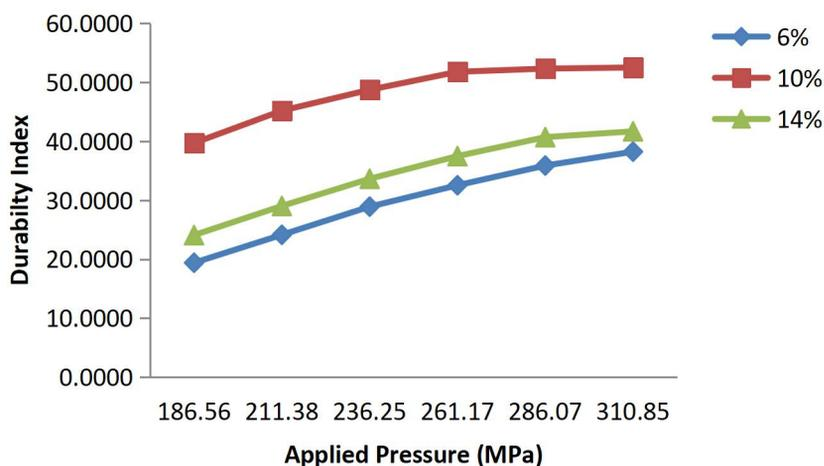
Figure 10: Effect of Applied Pressure on the Durability Index of the Densified Biomass for Sawdust at Different Moisture Contents
