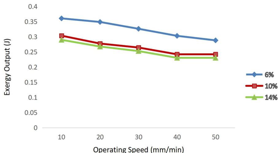
Figure 9: Effect of Operating Speeds on the Exergy Output of the Densification System using Huskdust at Different Moisture Contents
