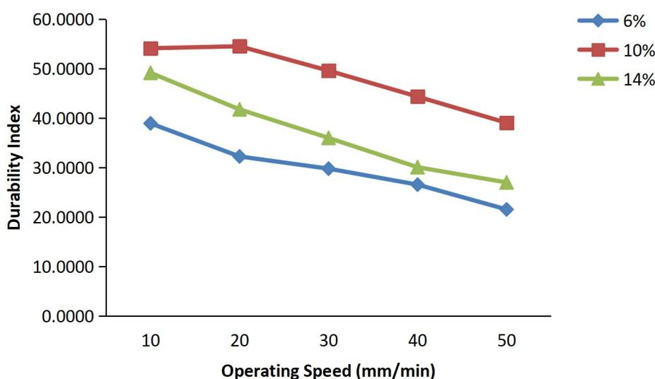
Figure 12: Effect of Operating Speed on the Durability Index of the Densified Biomass from Sawdust at Different Moisture Contents
