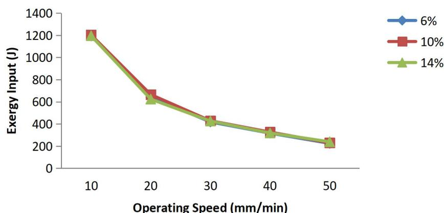
Figure 5: Effect of Operating Speed on the Exergy Input using Huskdust at Different Moisture Contents
