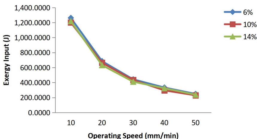
Figure 4: Effect of Operating Speed on the Exergy Input using Sawdust at Different Moisture Contents
