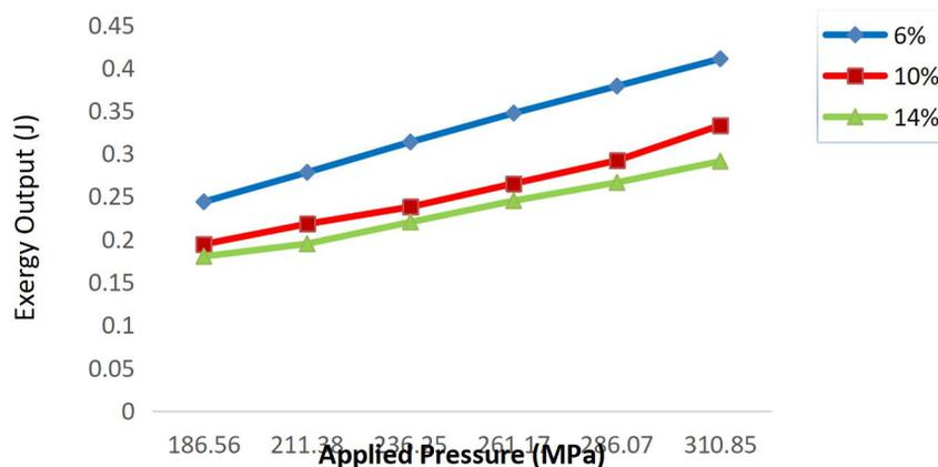
Figure 7: Effect of Applied Pressure on the Exergy Output of the Densification System using Huskdust at Different Moisture Contents
