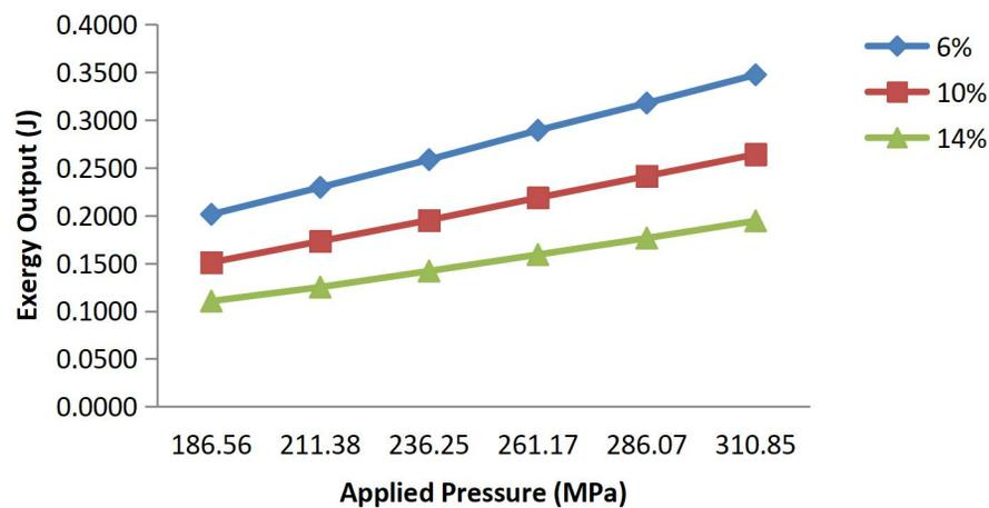
Figure 6: Effect of Applied Pressure on the Exergy Output of the Densification System using Sawdust at Different Moisture Contents
