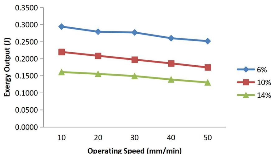
Figure 8: Effect of Operating Speeds on the Exergy Output of the Densification System using Sawdust at Different Moisture Contents
