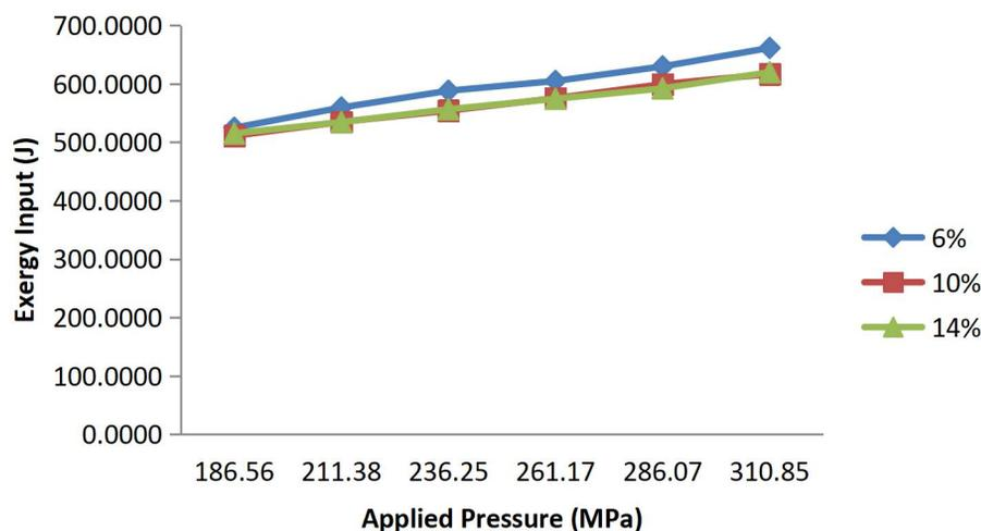
Figure 2: Effect of Applied Pressure on the Exergy Input using Sawdust at Different Moisture Contents
