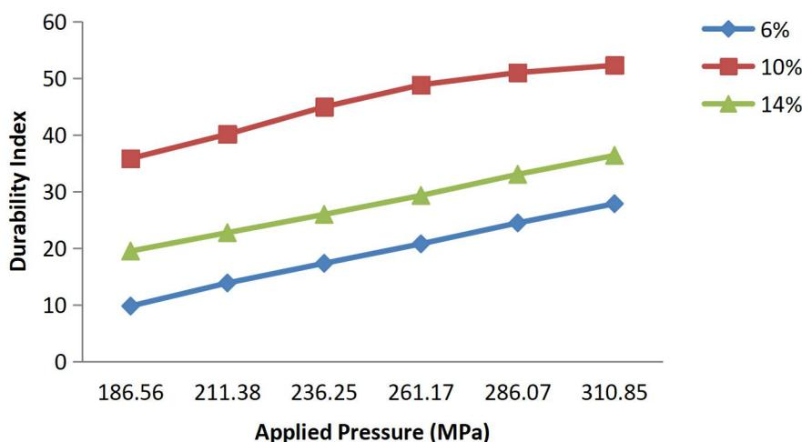
Figure 11: Effect of Applied Pressure on the Durability Index of the Densified Biomass for Huskdust at Different Moisture Contents
