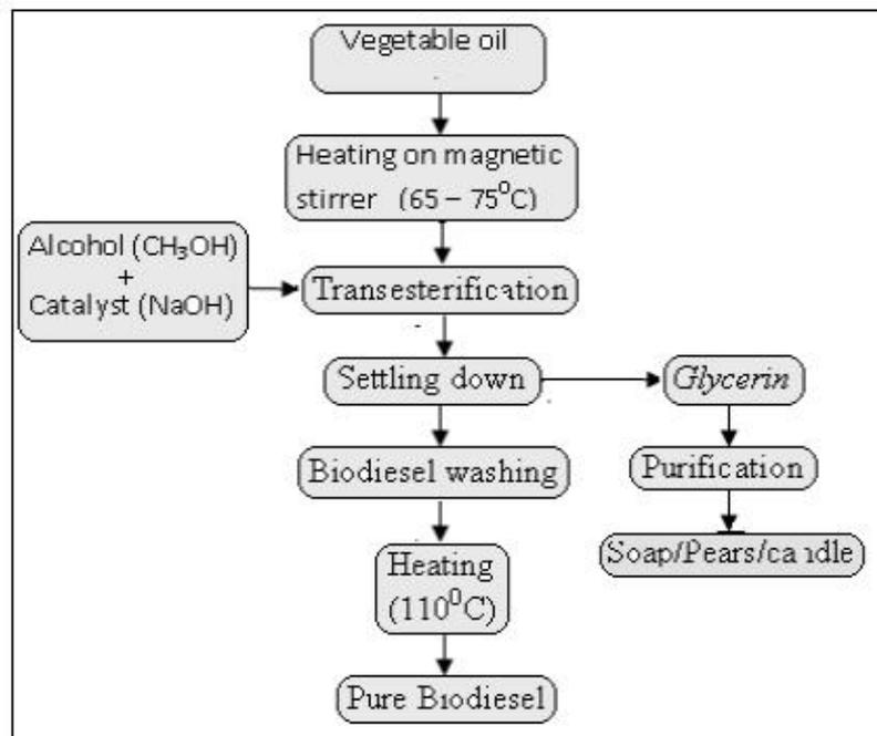
Figure 1: Biodiesel production process flowchart (Jadhav et al. 2016)
