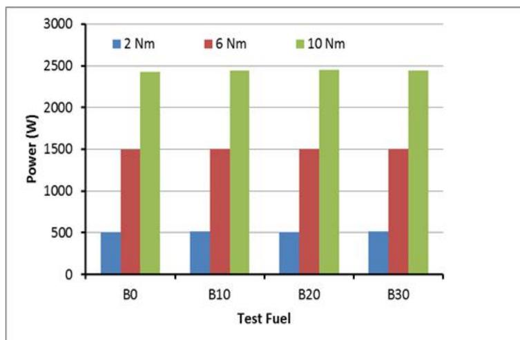
Figure 4: Brake Power of diesel and blends at different torques
