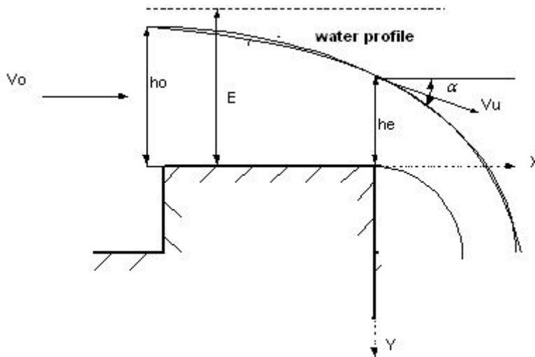
**Figure 1: Schematic diagram of free overfall water profile passing over hydraulic structure**
