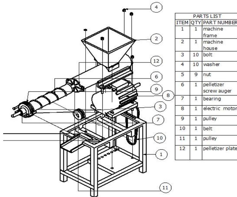
Figure 2: Exploded view Drawing of Fish Feed Pelletizing Machine
