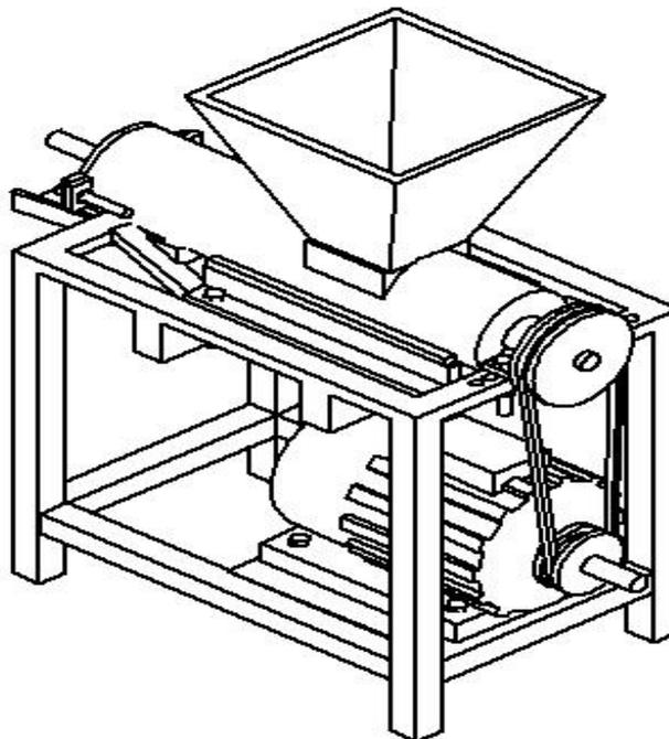
Figure 1: Isometric View of Fish Feed Pelletizing Machine
