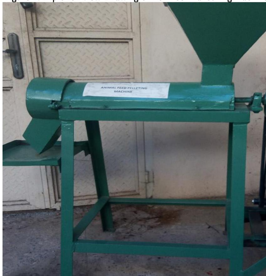
Figure 3: Modified Fish Feed Pelletizing Machine
