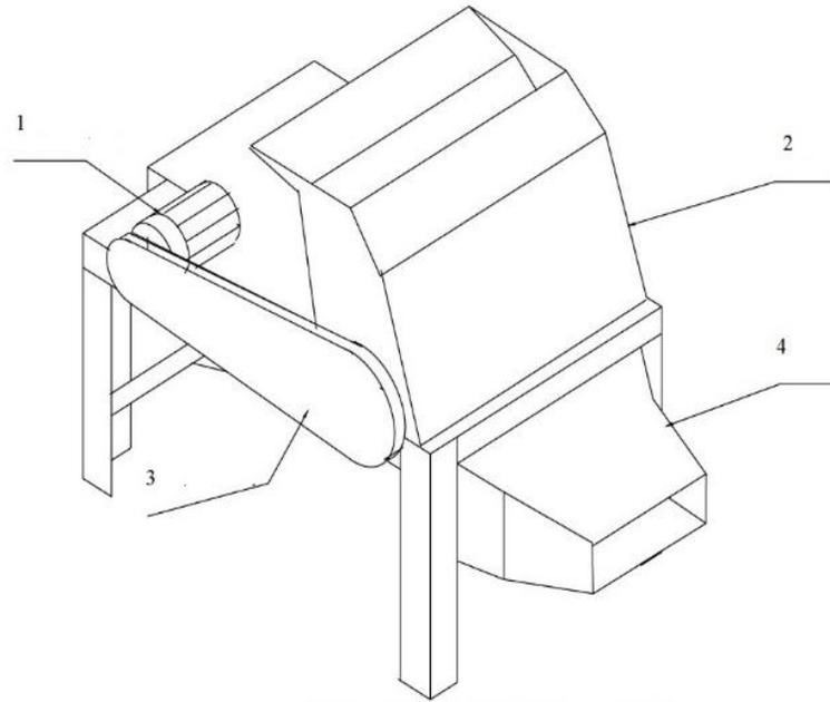
Figure 1a: Waste Shredding Machine Assembly
