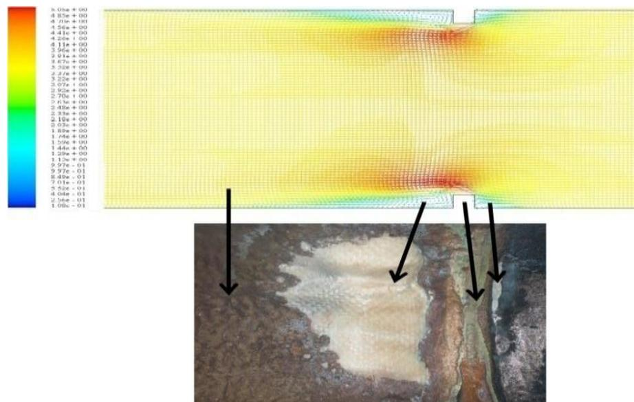
Figure 4: Finite element analysis of the inner pipe showing the orifice effect and the eddy zone near the backing bar correlated with the actual leaks on the inlet pipe.
