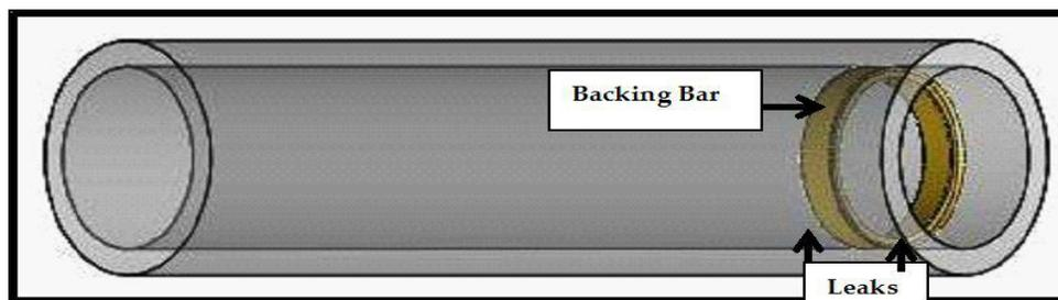
Figure 1: Big and small leak near the backing bar at about 6 o'clock position viewed from the inner side of seawater inlet pipe.
