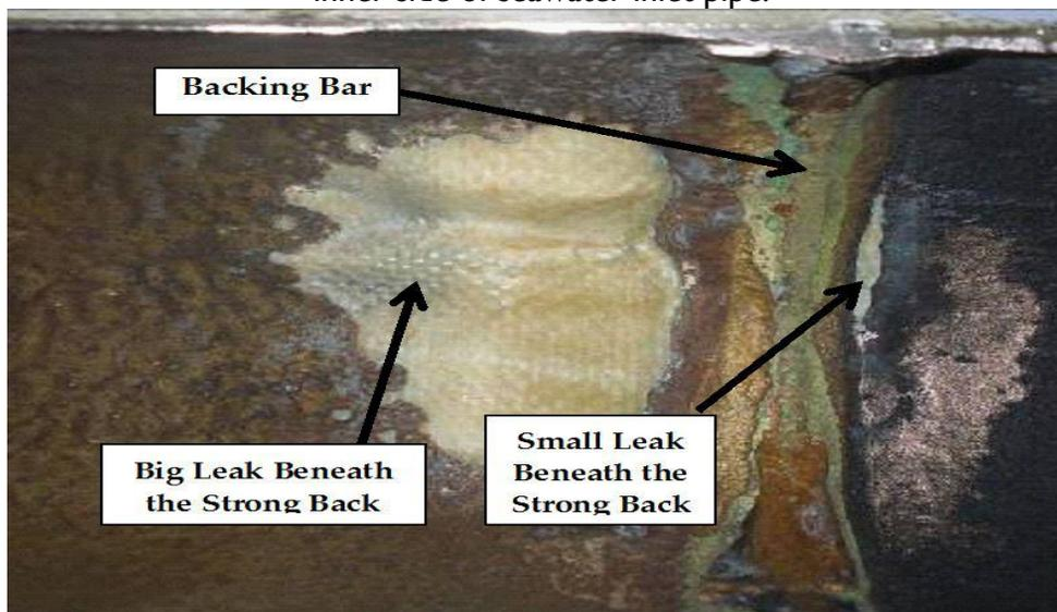
Figure 2: Big and small leak near the backing bar at about 6 o'clock position viewed from the inner side of seawater inlet pipe.
