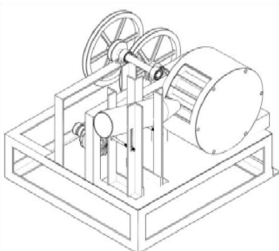
Figure 6: Isometric View of the Cross Flow Turbine.
