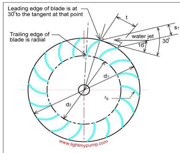
Figure 5: Critical geometry of the cross-flow turbine.
