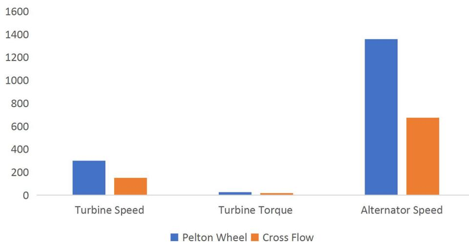
Figure 13: Comparing the Mean Output from the Two Turbines
