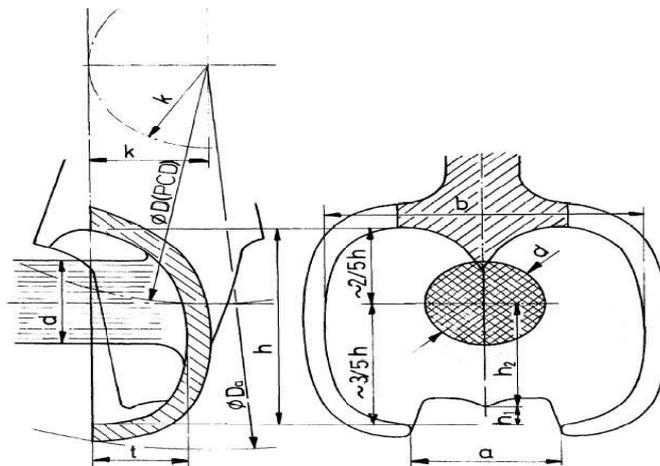
Figure 4: Ideal Dimensions of a Pelton Wheel.
