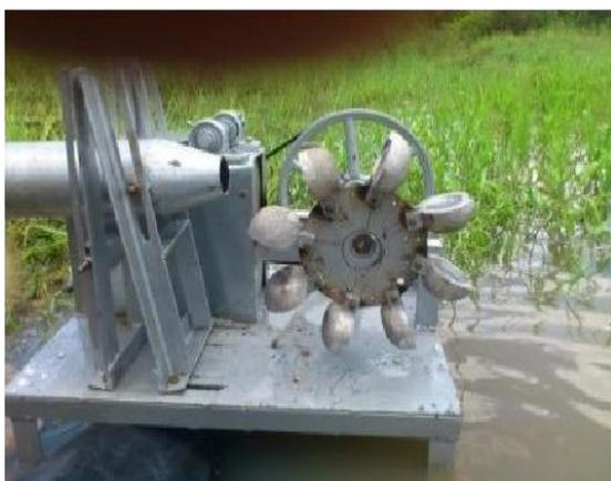
Figure 11: Pictorial View of the Pelton Wheel Turbine
