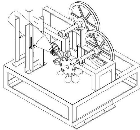
Figure 7: Isometric View of the Pelton Wheel Turbine.
