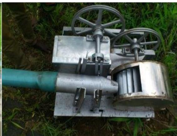
Figure 12: Pictorial View of the Cross Flow Turbine
