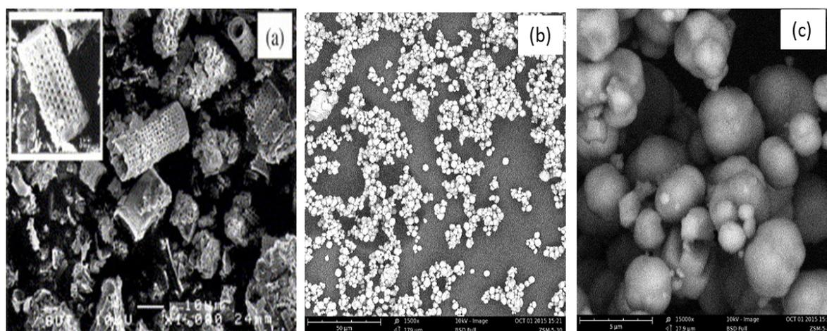
Figure 3: SEM images for (a) raw diatomite, (b) ZSM-5 from diatomite at low magnification (c) ZSM-5 from diatomite at high magnification.
