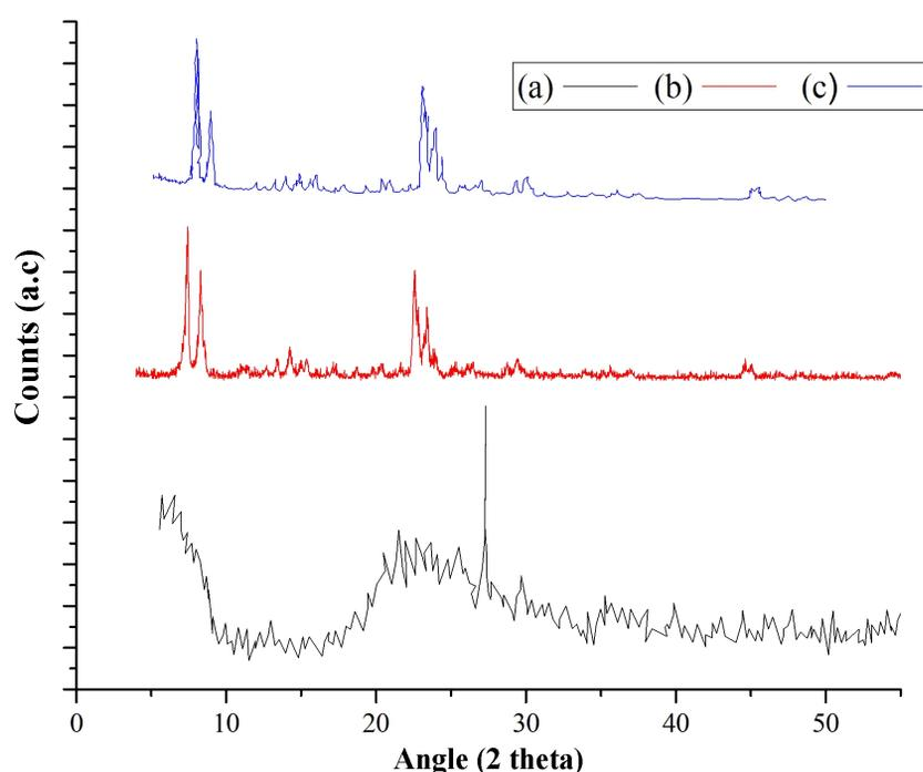
Figure 1: XRD pattern of (a) Diatomite (b) diatomite based ZSM-5 and (c) Reference ZSM-5
