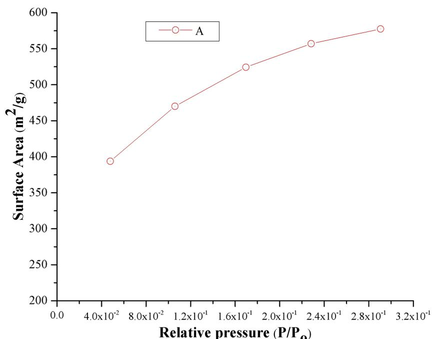
Figure. 4: N<sub>2</sub> Adsorption-desorption Isotherms of the Synthesized ZSM-5 from Bularafa Diatomite
