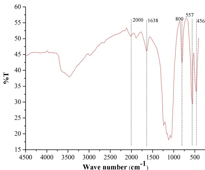
Figure 2: FTIR spectra for Bularafa diatomite based ZSM-5
