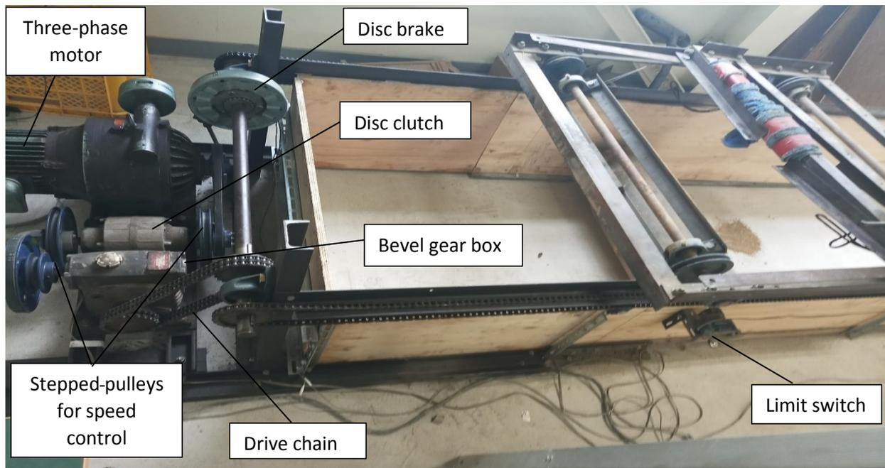
Figure 2: Control and power unit of the soil bin
