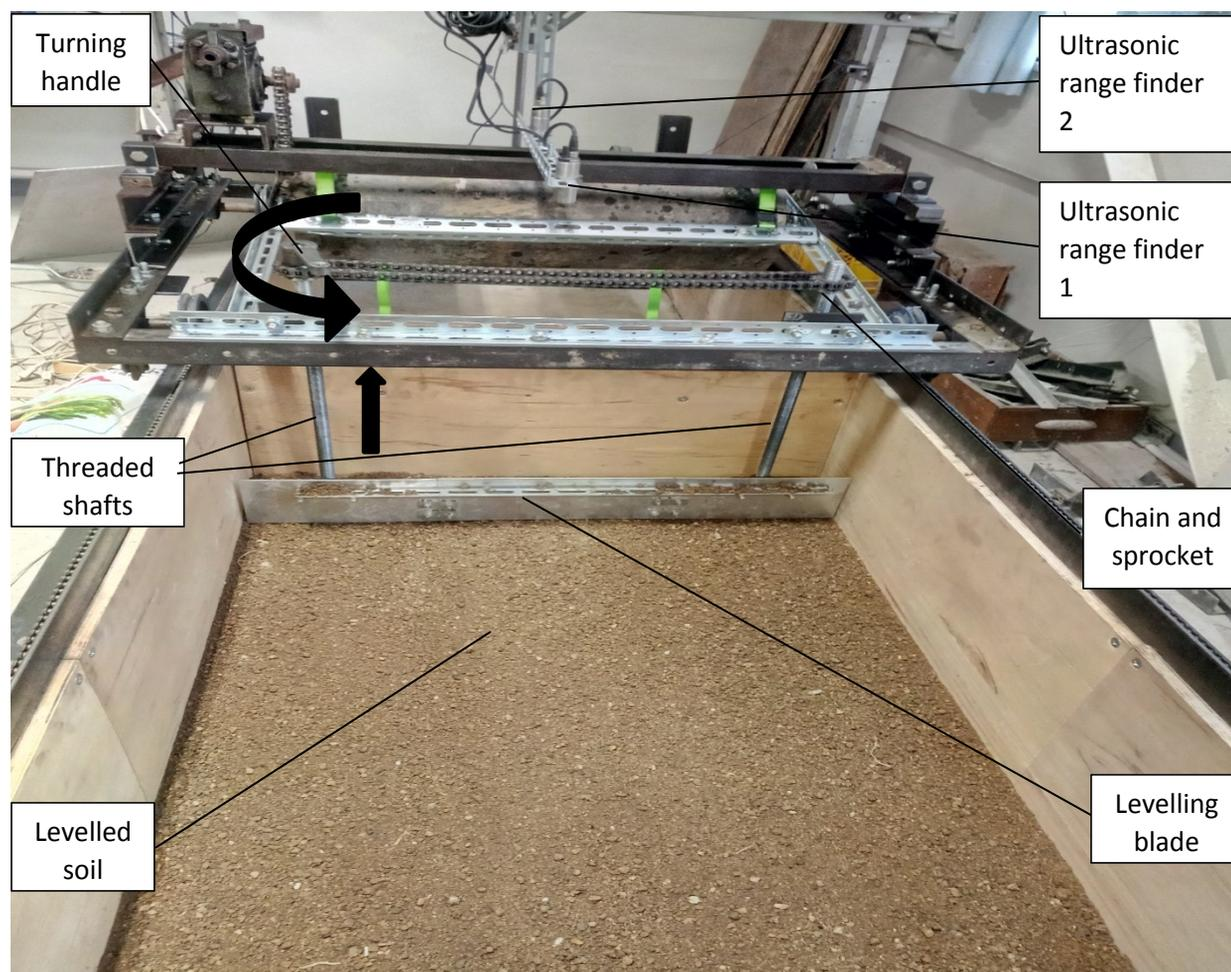
Figure 3: An already levelled soil and the stepless leveler fixed on one of the carts
