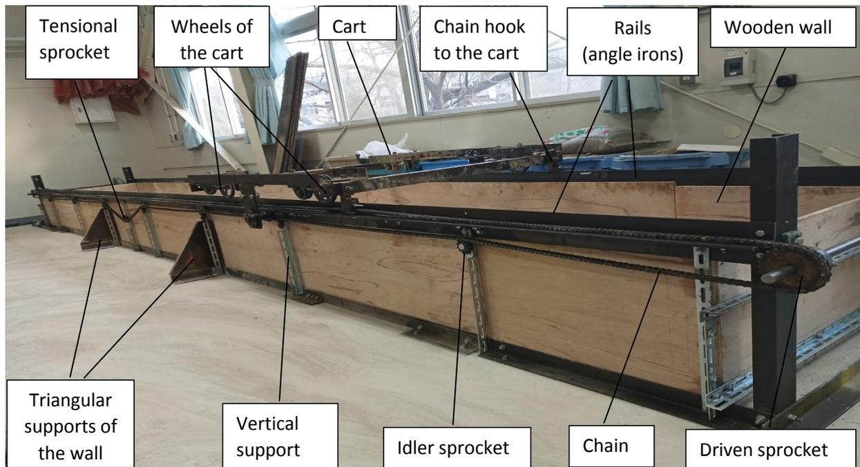
Figure 1: Pictorial view of the soil bin
