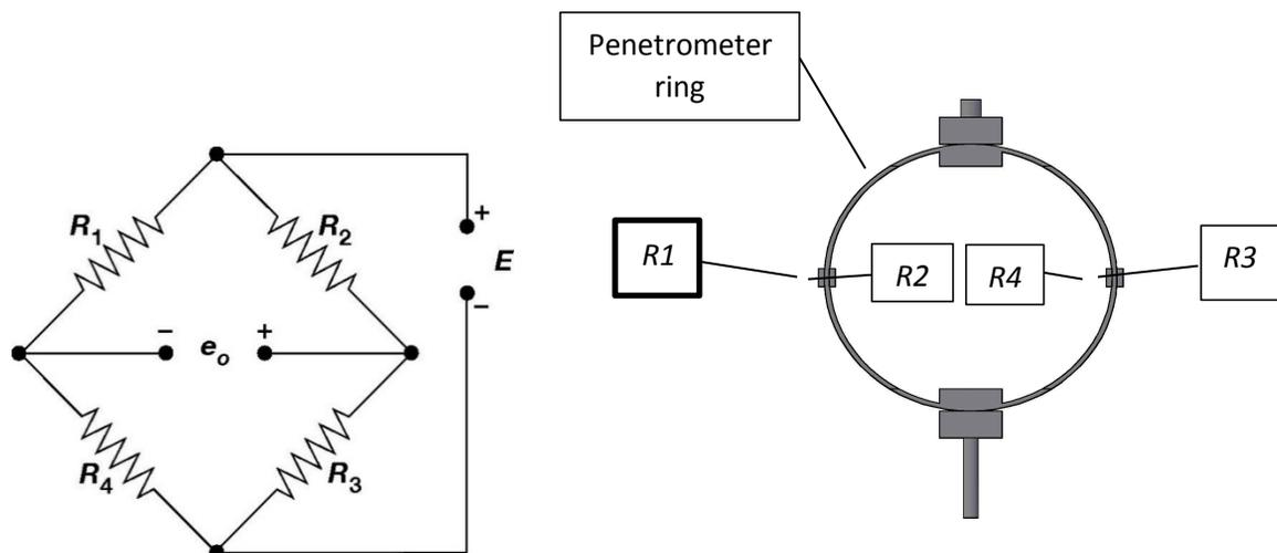
Figure 4: Position of the strain gauges on the penetrometer ring and the circuit diagram for the strain gauges connection
