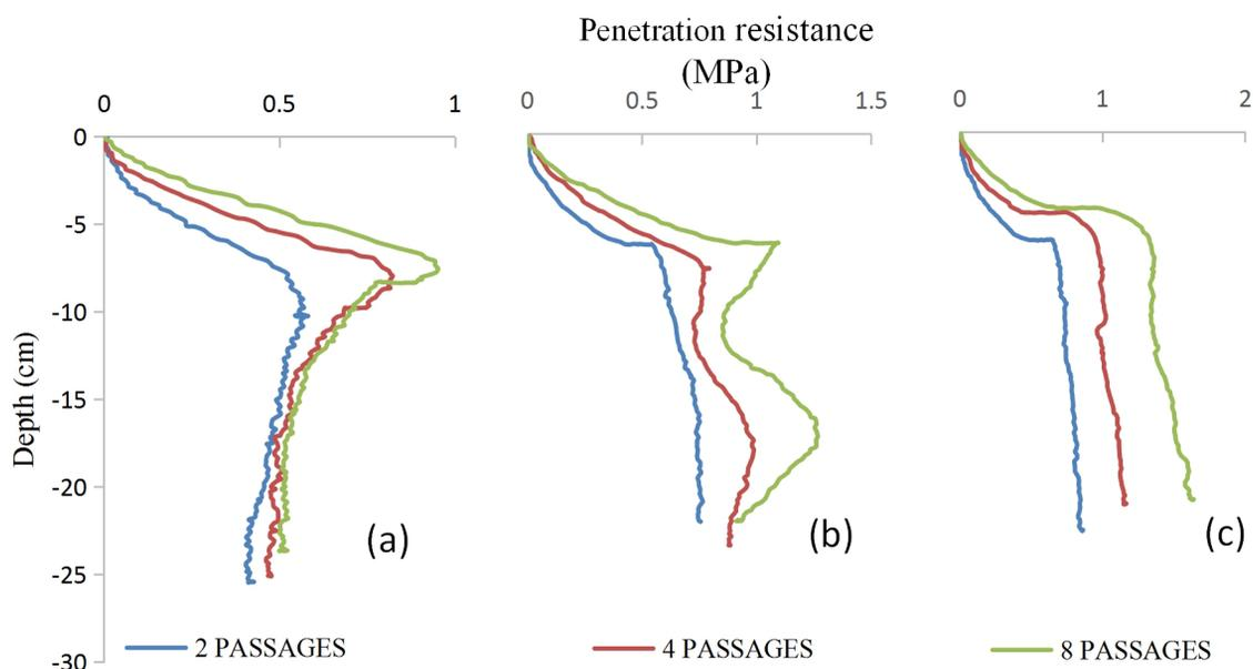
Figure 6: Variations in cone penetration resistance with depth, resulting from different number of layers and passages of the roller: (a) 1-layer, (b) 2-layer and (c) 4-layer experiments
