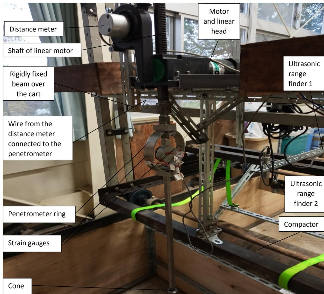
Figure 5: Pictorial diagram showing the digitized penetrometer and other components.
