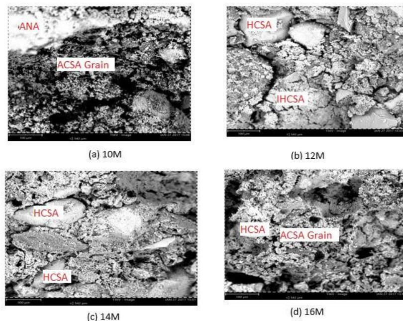
Figure 7: SEM images of AACSAM at 28 days of hydration with different NaOH concentrations.
