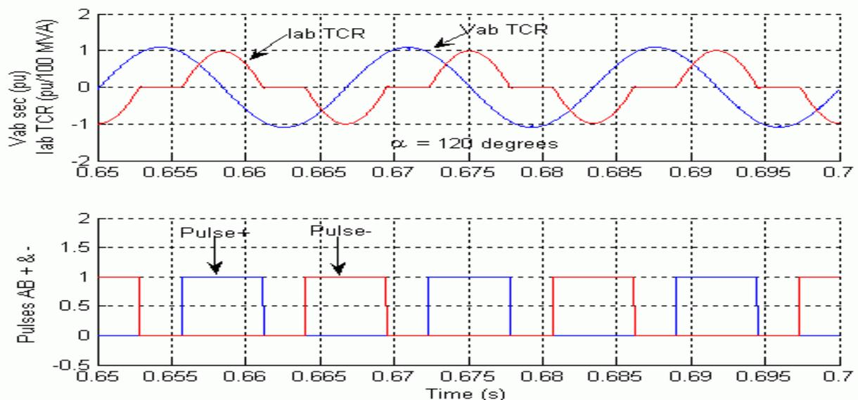
Figure 8: Steady-State Voltage and Current in TCR AB
