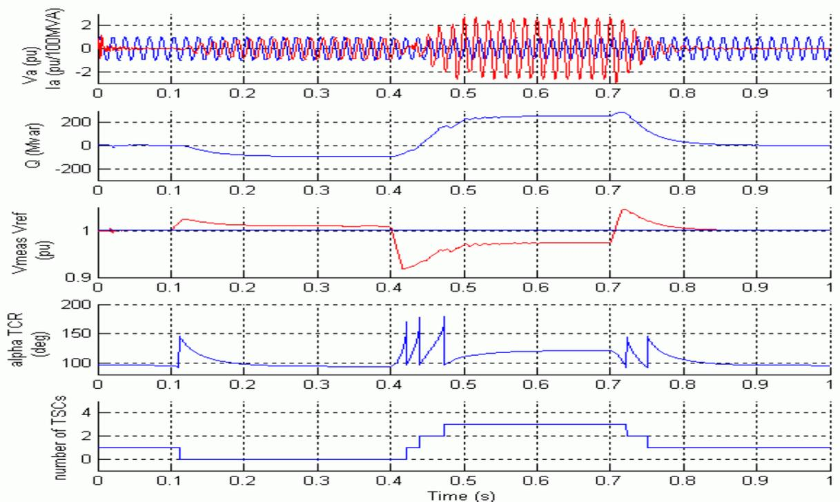
Figure 7: Waveforms Illustrating SVC Dynamic Response to System Voltage Steps
