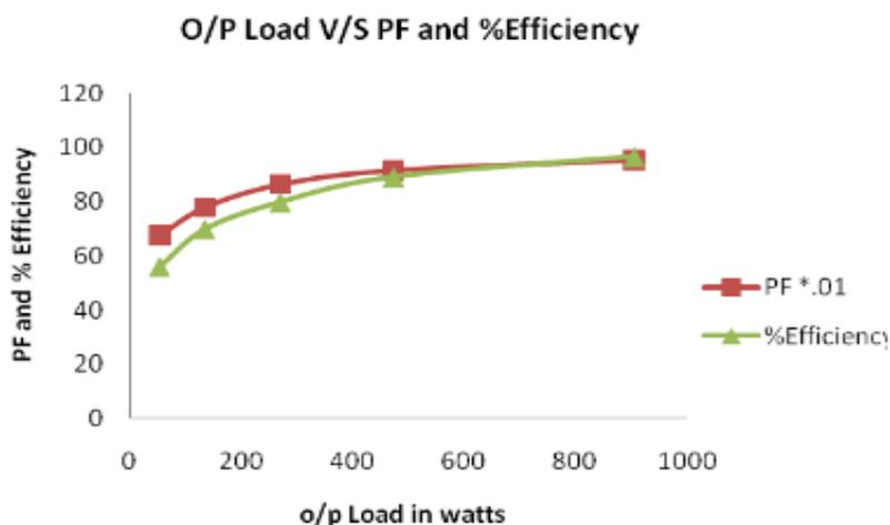
**Figure 10:** Power Factor and % efficiency V/S output load in watt
