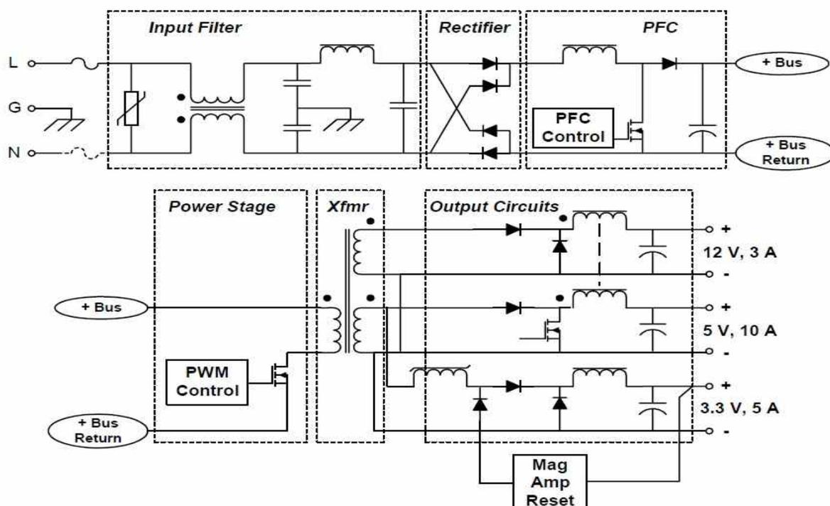
Figure 2: Circuit Diagram of Forward Converter using PFC Control
