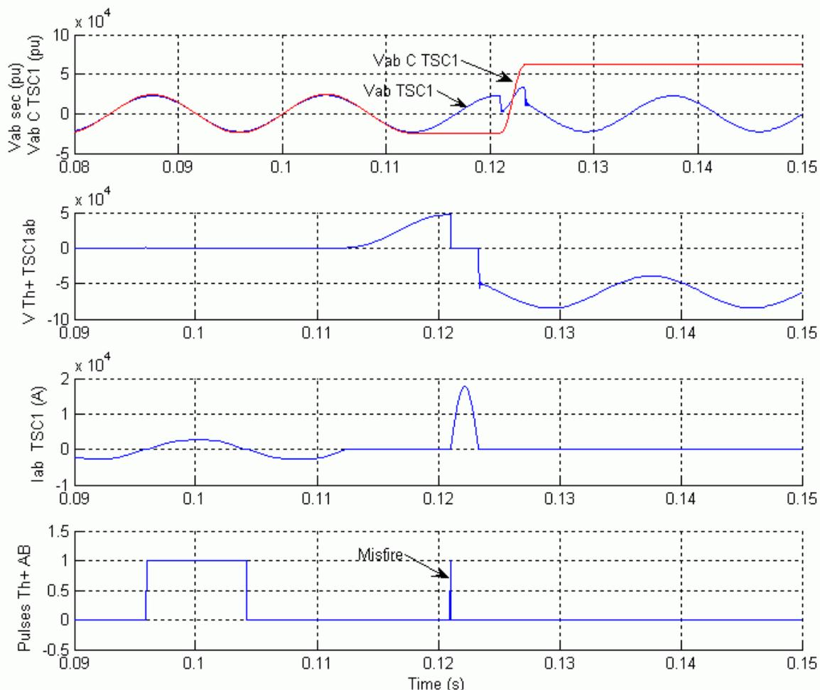
**Figure 9:** TSC Voltages and Current Resulting from Misfiring on TSC1
