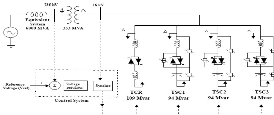
**Figure 4:** Single-line Diagram of a Static Var Compensator and Its Control System
