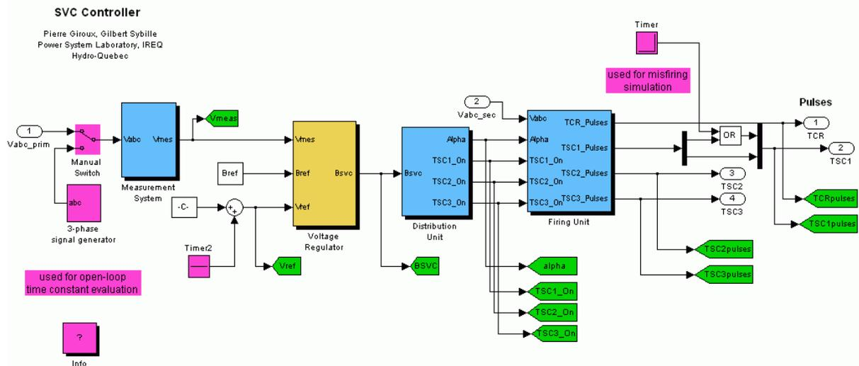
Figure 6: Simulink Models of SVC Controller
