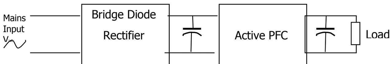
Figure 1: Block Diagram of AC-DC Converter with PFC
