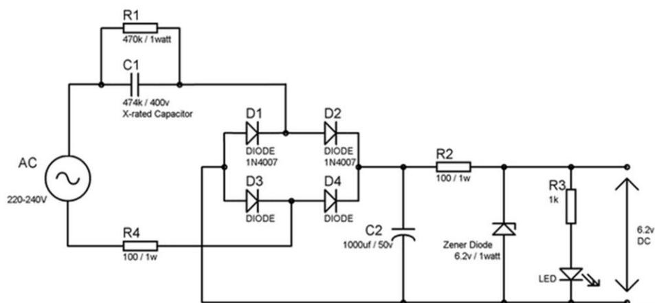
**Figure 3:** Conversion of an AC to DC and Stepping down the Voltage without Transformer
