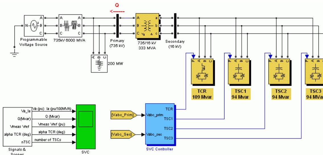
**Figure 5:** SPS Model of the 300 Mvar SVC
