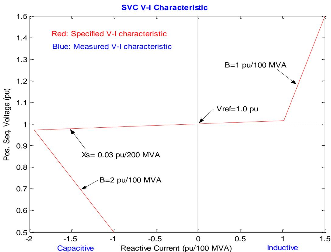
**Figure 11:** Voltage – Ampere Characteristics
