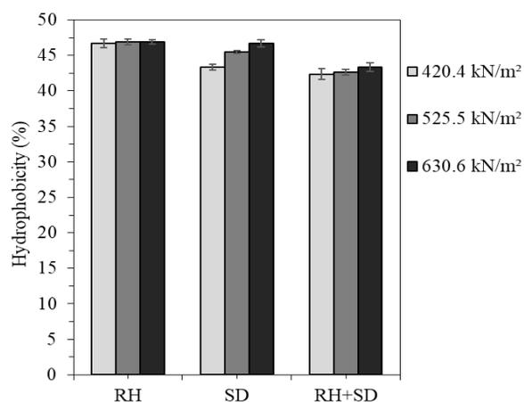
**Figure 7:** The hydrophobicity of the produced briquettes
