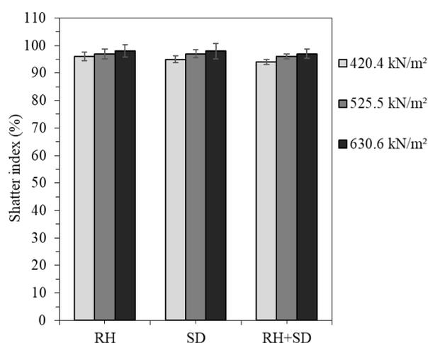
**Figure 6:** The shatter index of the produced briquettes
