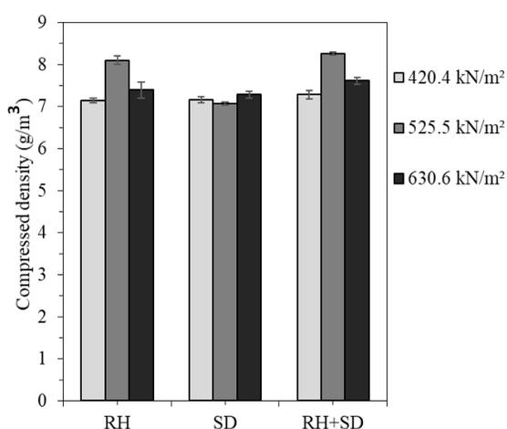
**Figure 5:** Compressed density of the produced briquettes
