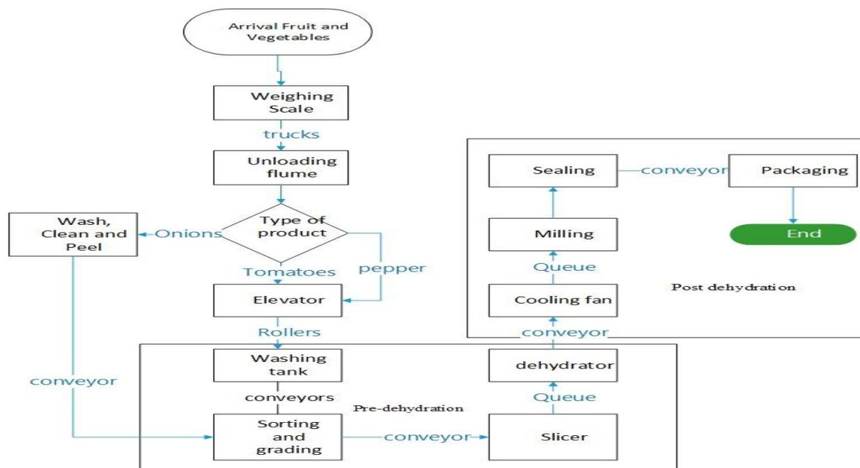
**Figure 3:** Proposed process flowchart for dehydration of fruit and vegetables processing plant.
