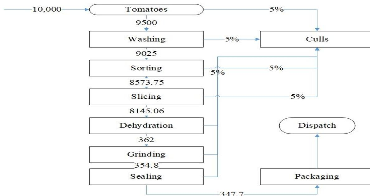
**Figure 4:** The simplified process block diagram (PBD) for dehydration of tomatoes
