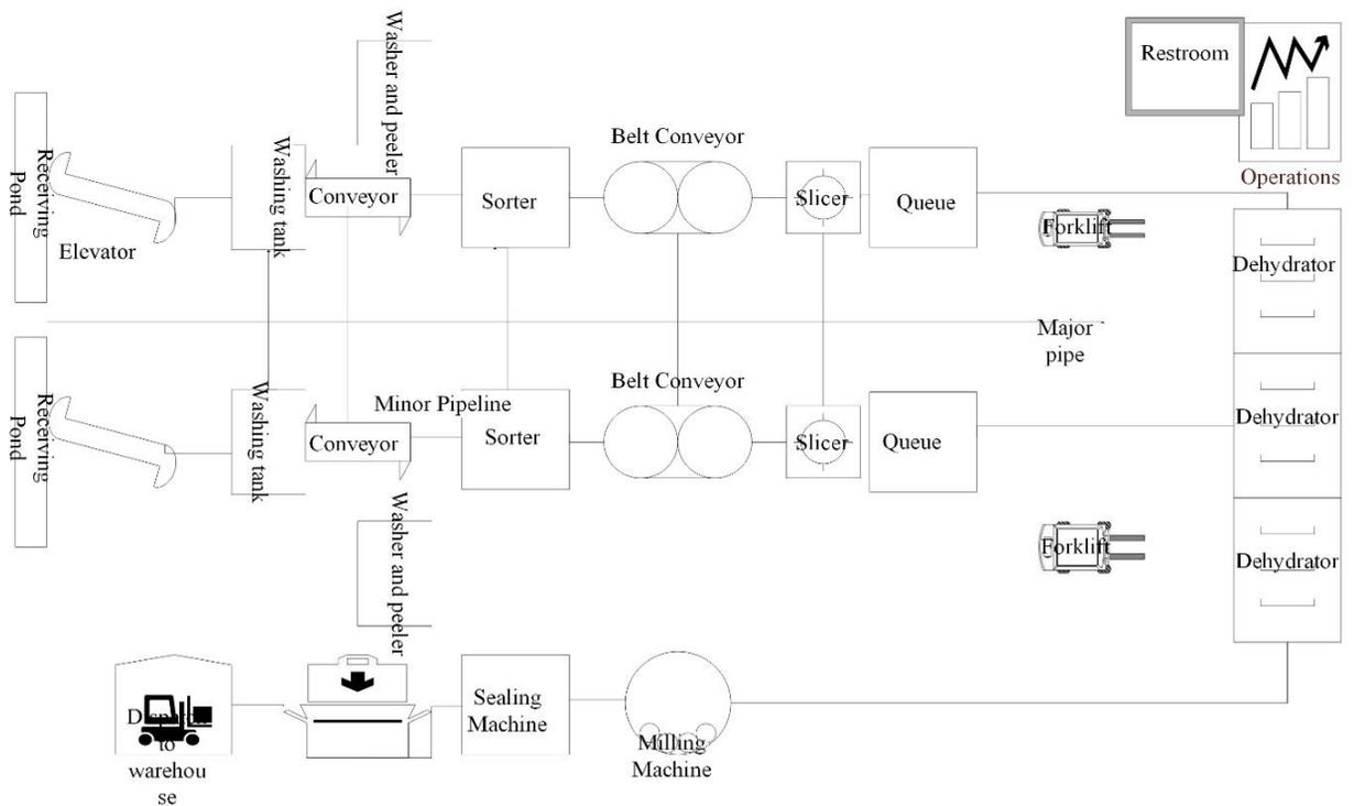
**Figure 8:** Floor plan for processing of dehydrated fruit and vegetables
