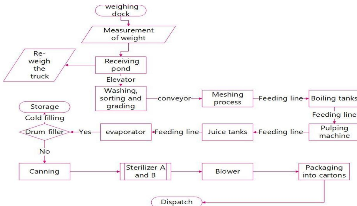
Figure 1: Process flow chart of tomato paste production at Savannah Integrated Export Processing Farms©
