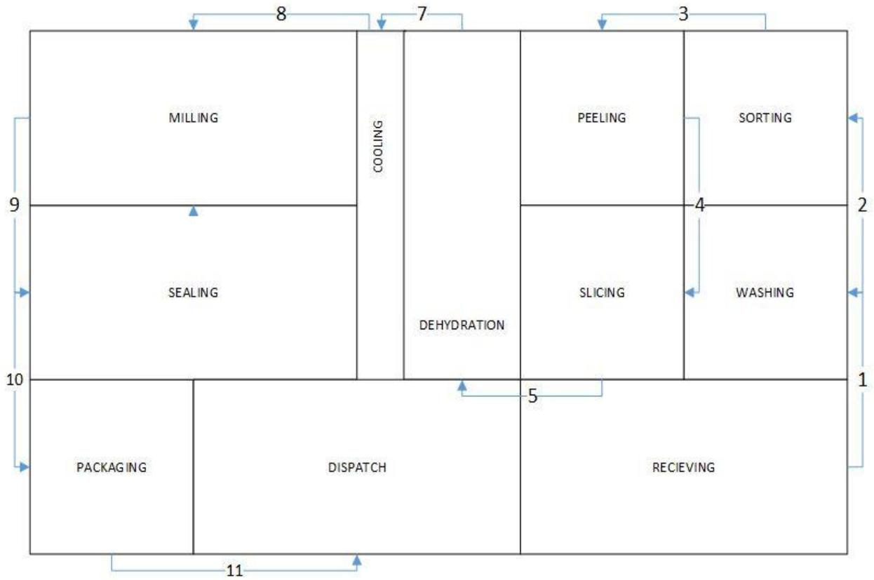
**Figure 7:** Dimensionless block diagram for the proposed process layout
