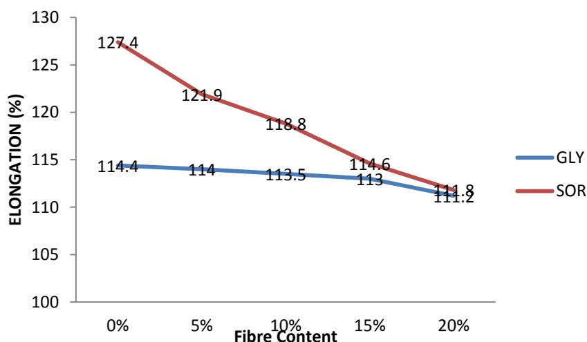
**Figure 3:** Effect of fiber content on elongation at break of biocomposite.
