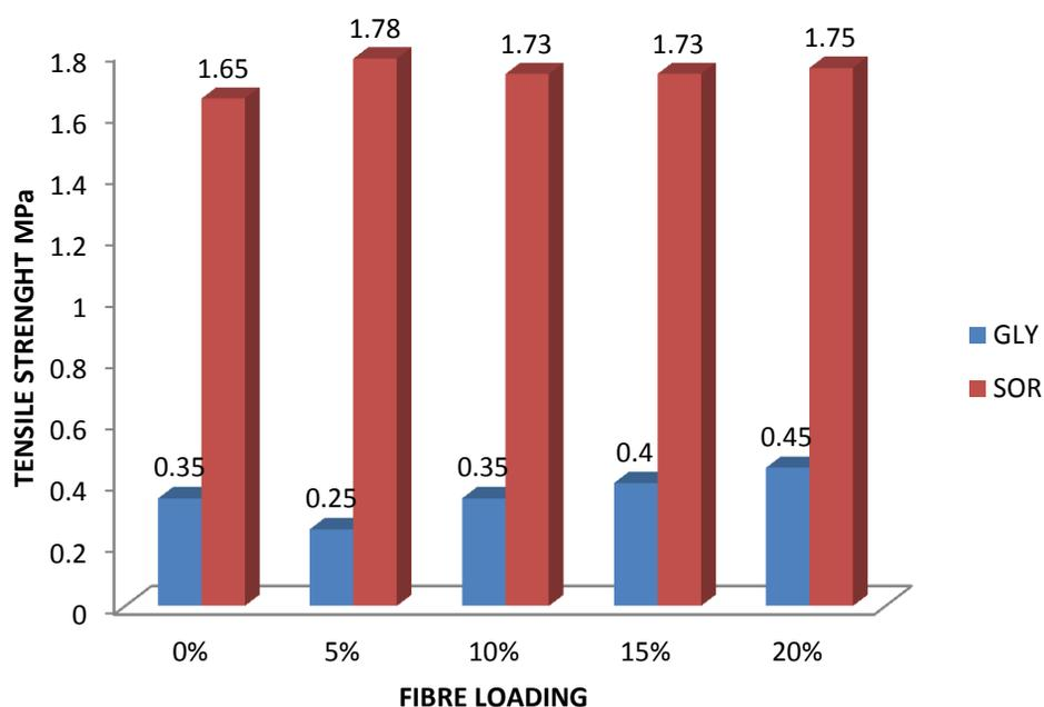
Figure 2: Variation of Tensile Strengths of produced bio-composite with Fibre Loading.
