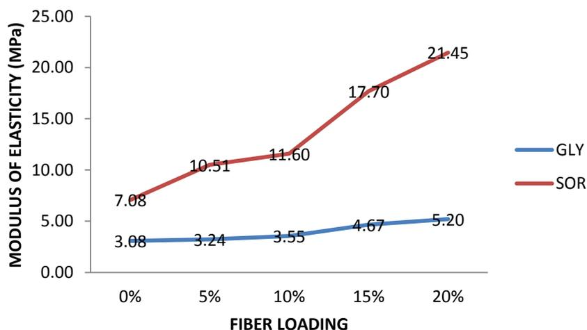
**Figure 2:** The effect of fibre loading on the Modulus of Elasticity of Corn-Plasticized Biocomposite.
