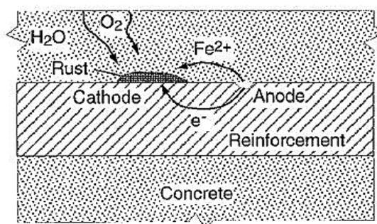
Figure 1: Corrosion formation in concrete (Carino, 1999)
