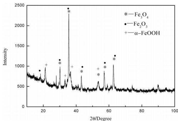
Figure 9: Typical XRD response spectra for corrosion (Liu et al., 2017)
