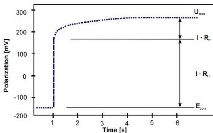
Figure 3: Electrochemical potential of steel against time (Sørensen and Frølund, 2002)
