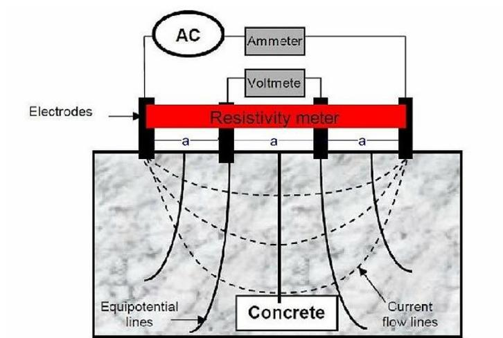
Figure 11: Wenner four-probe device measuring concrete resistivity (Carino, 1999)
