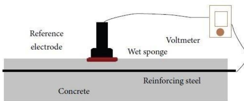
Figure 6: Typical half-cell potential set-up (Verma et al., 2014)
