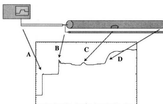
Figure 7: Pit corrosion monitored by time-domain reflectometry Curve (Liu et al., 2001)
