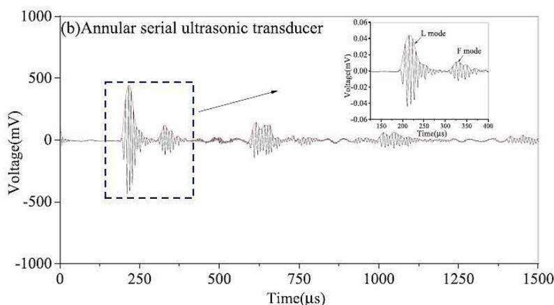
Figure 8: Typical ultrasonic time-domain spectra response (Liu et al., 2019)
