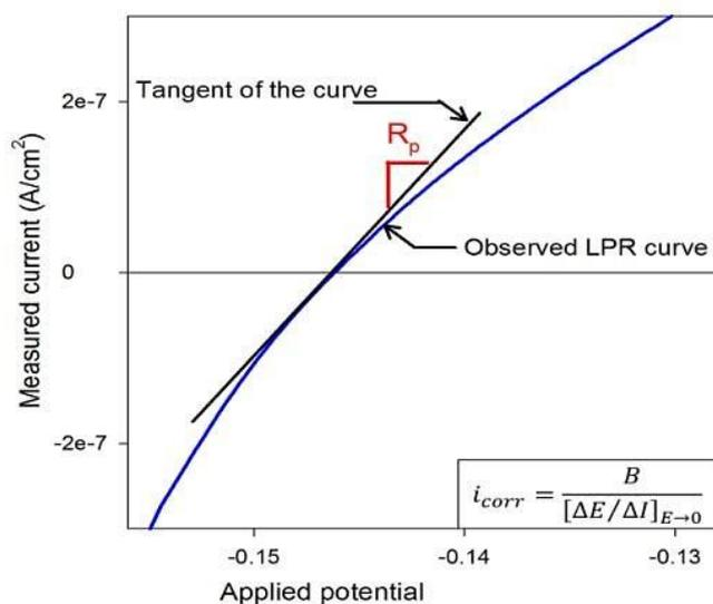
Figure 5: Typical polarization resistance curve (Karuppanasamy and Pillai, 1995)
