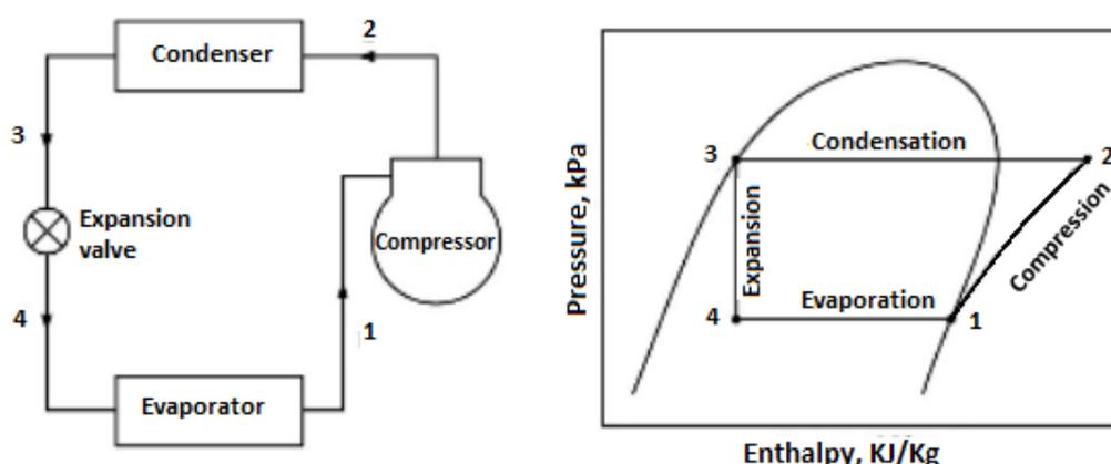
Figure 1: Schematic diagram of refrigeration system with enthalpy-pressure relation (Nasution et al., 2019)
