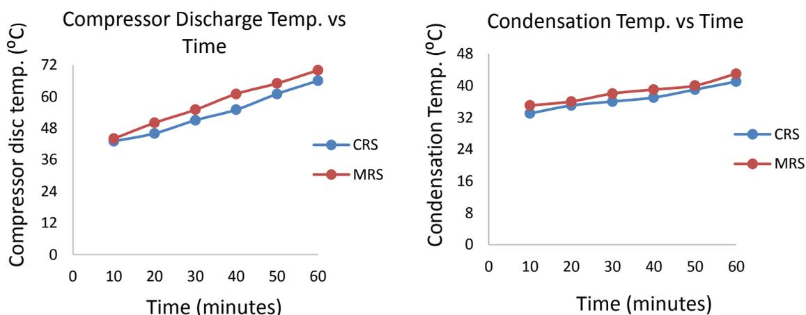
**Figure 5:** Comparison of compressor discharge and condensation temperature with time
