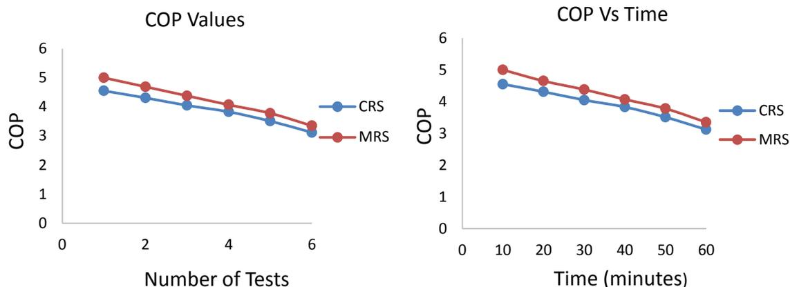
**Figure 3:** Comparison of COP for the conventional and modified refrigeration systems
