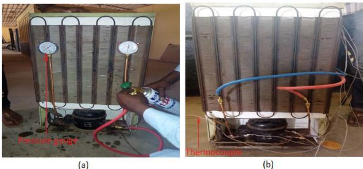
Figure 2: Pressure gauges (a) and thermocouples (b) fixed to the refrigerator to obtain data
