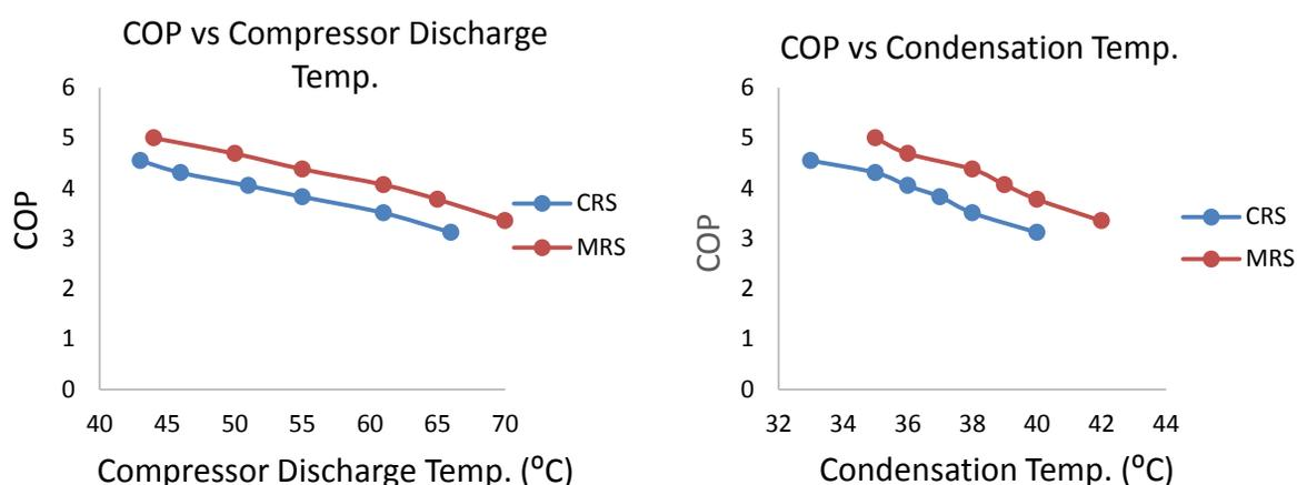
**Figure 4:** Comparison of COP with compressor discharge and condensation temperature
