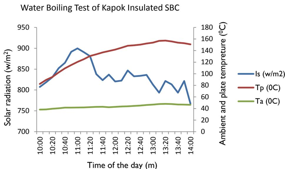
Figure 5: Variation of Water Temperature with Corresponding Solar Radiation and Ambient Temperature
