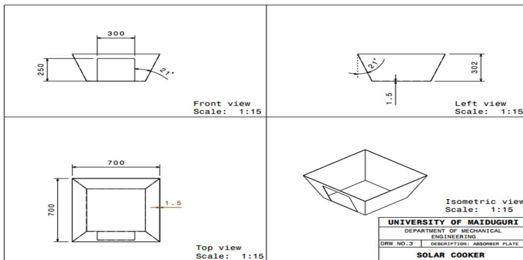
Figure 2: isometric view of solar box absorber plate
