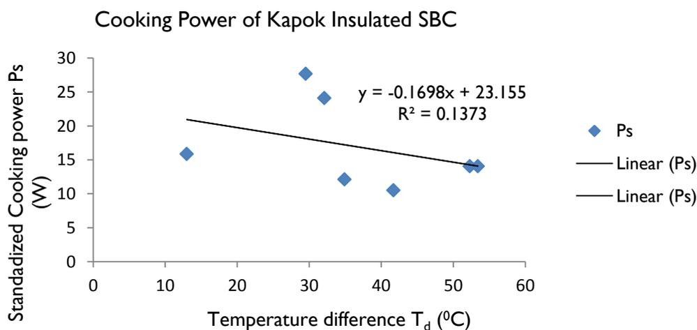
Figure 6: Variation of Standard Cooking Power with Corresponding Temperature Difference
