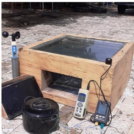
Figure 3: Constructed solar box cooker and instrumentation
