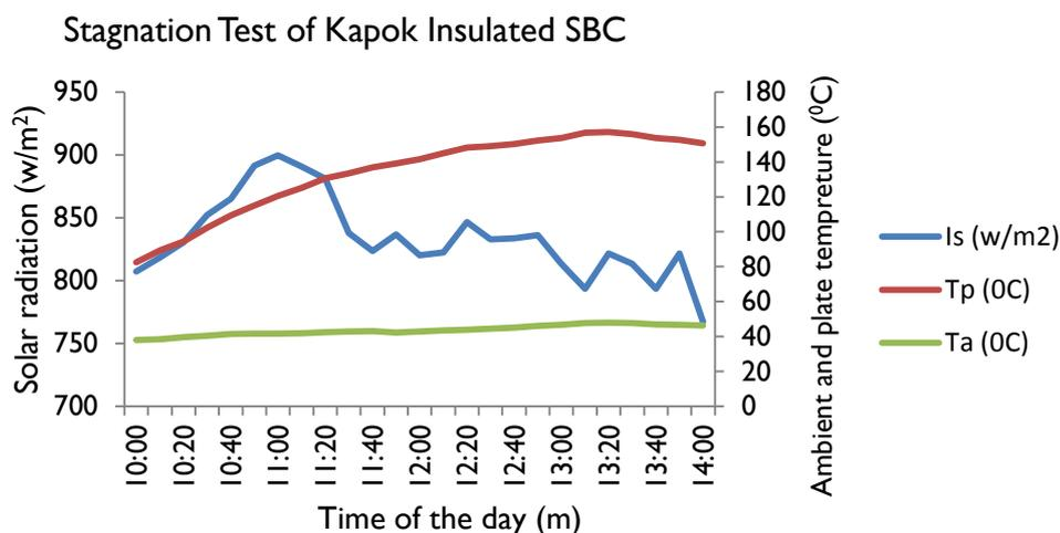
Figure 4: Variation of Absorber Plate Temperature with Corresponding Solar Radiation and Ambient Temperature
