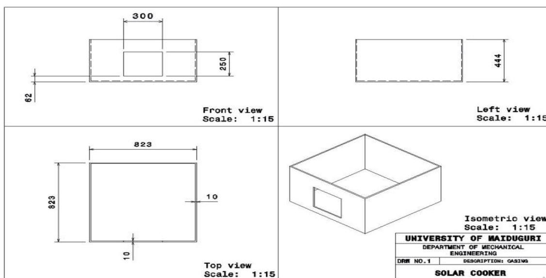
Figure 1: isometric view of solar box casing
