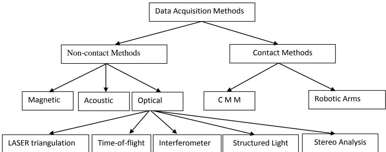
Figure 1: Classification of data acquisition techniques used in contact and non-contact approaches for three dimensional systems.
