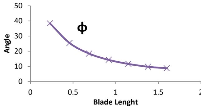
Figure 7: Blade Setting Angle
