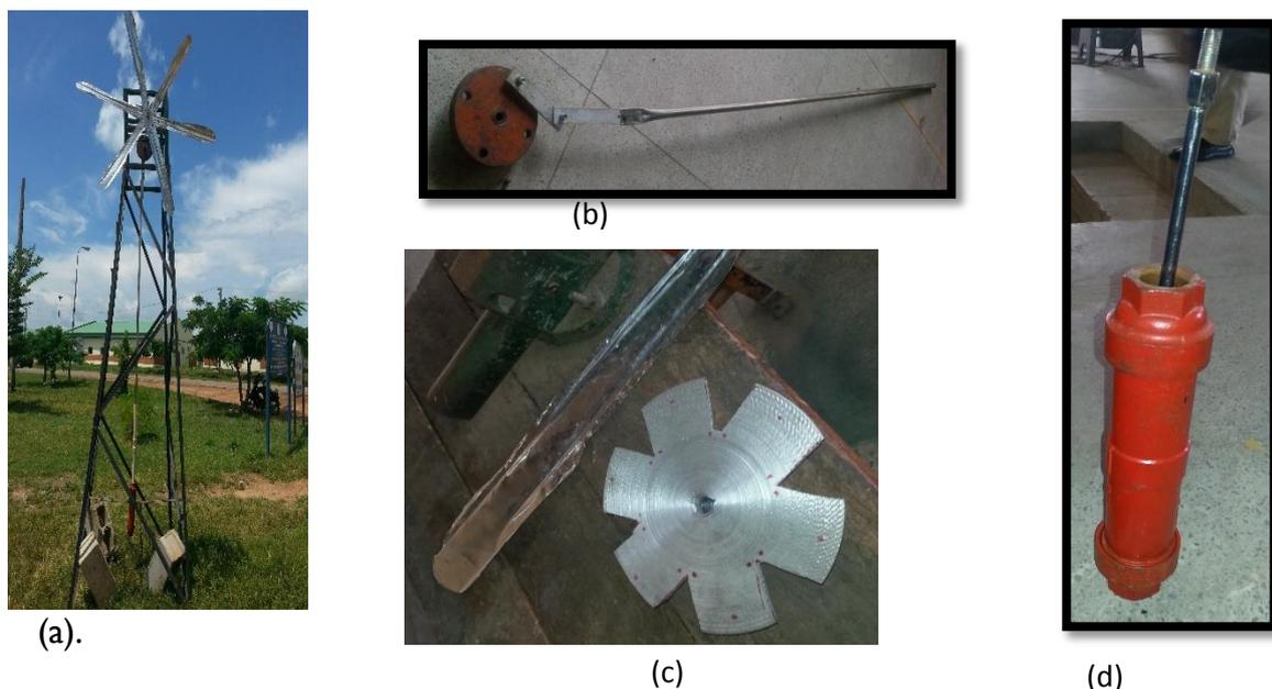
Figure 6: Fabricated Components, (a) Assembled Windmill (b) Flywheel and Links Mechanism. (c) Blade and Hub, (d) Positive Displacement Pump.
