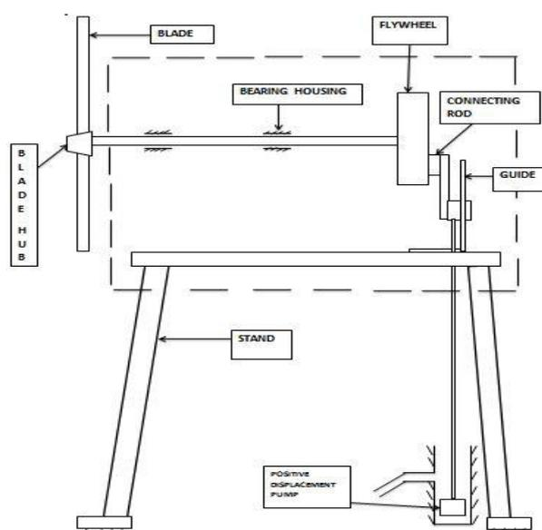
Figure 1: Schematic Diagram of the Windmill Water Pump.
