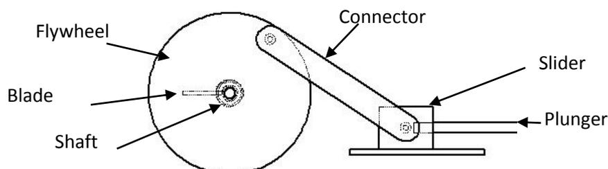
Figure 5: Modified Slider-Crank Mechanism.
