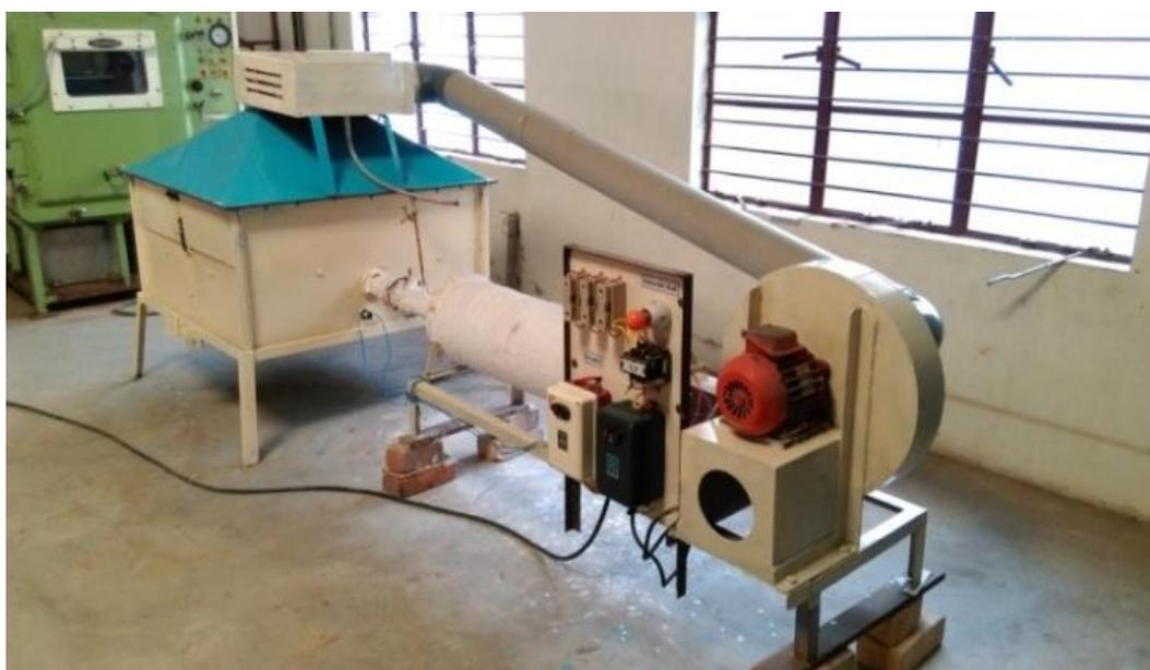
Figure 4: Flat-bed Dryer fitted with HRU
