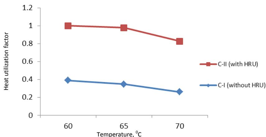
Figure 6: Heat utilization factor at different operating conditions
