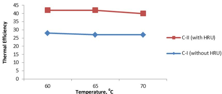
Figure 7: Overall thermal efficiencies at different operating conditions
