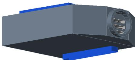
Figure 1: Conceptual view of Heat Recovery Unit
