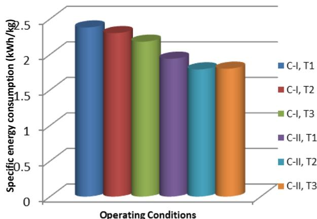
Figure 8: Specific energy consumption at different operating conditions
