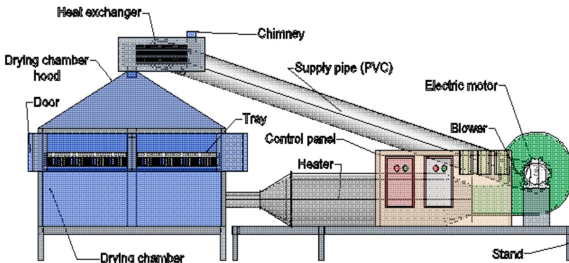
Figure 3: Conceptual front view of Flat-bed dryer with HRU
