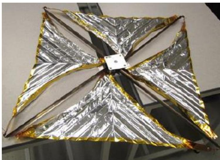
Figure 3 Deployed Cranfield DOM (Taylor, 2013)
